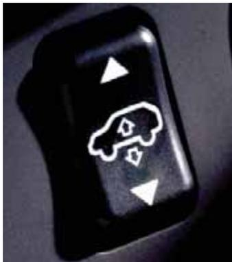
The available four-wheel air-suspension system offers four modes (High, Normal, Low and Access) and can automatically vary its height based on vehicle speed and engine status. For example, the system can provide increased ground clearance one moment and improved aerodynamics for performance driving the next. In some cases, automatically, to help lessen wind resistance. When parked, the RX conveniently assumes its lowest point for easier passenger and cargo loading.
