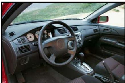
Instruments and controls are very well laid out, but only the driver's power window control is lit up at night. The heating system works fairly quickly, but the air distribution between floor and windshield could be better, or at least easier to adjust. With the lever in the Heat/Defrost position, there is too little air or heat at floor level. The rear defroster elements should cover a bigger area of the window.
