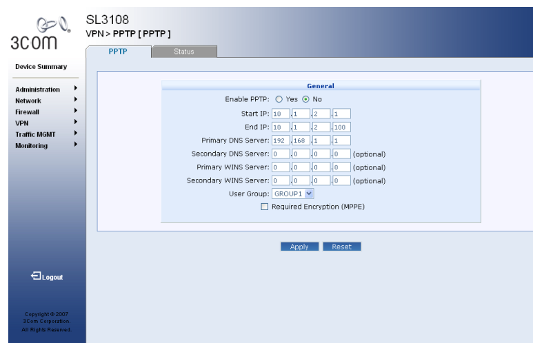
Figure 16.1. PPTP Server Configuration Page
