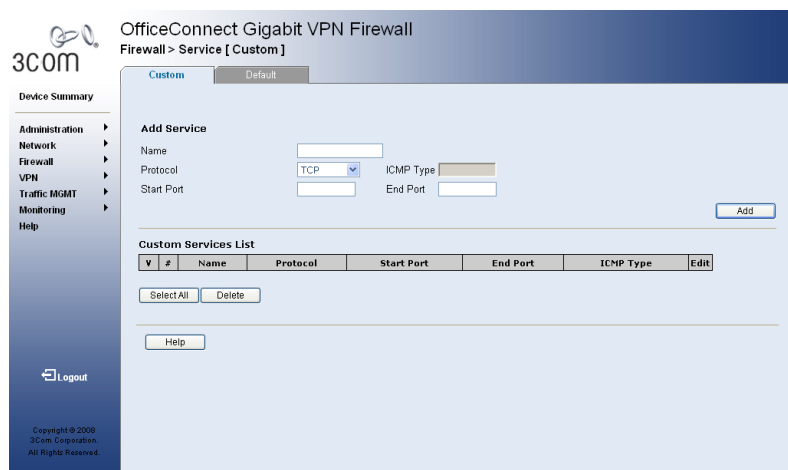
Figure 11.11. Service List Configuration Page
