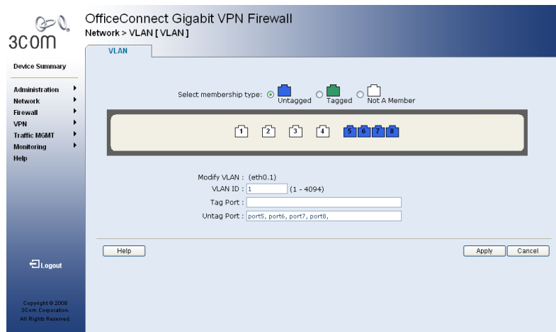
Figure 6.2 VLAN Configuration Page
