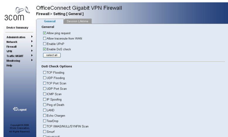
Figure 11.12. DoS Configuration Page
