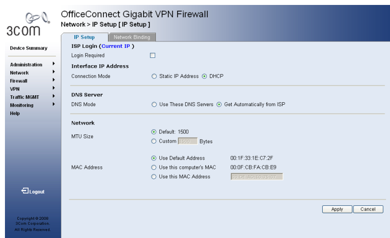
Figure 8.2 WAN Dynamic IP (DHCP client) Configuration Page
