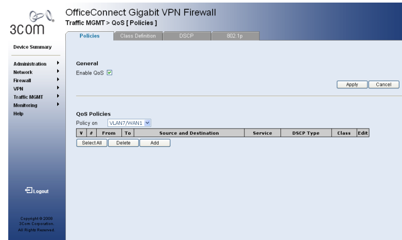
Figure 12.3 QoS Configuration Page
