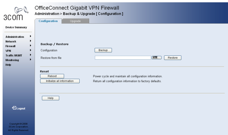
Figure 17.6. Default Setting Configuration Page
