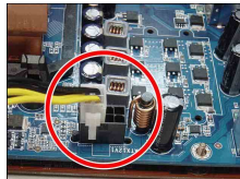
Plugged from a 4-pin ATX12V power.
