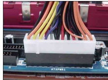
Plugged from a 24-pin ATX12V power.
