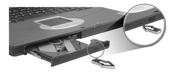
When the power is off, you can eject the drive tray using the emergency eject hole. See page 50.
