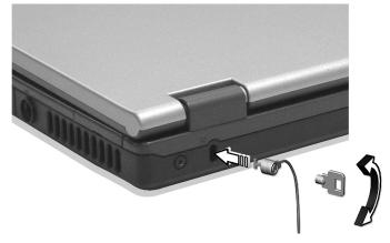
Wrap a computer security lock cable around an immovable object such as a table or locked drawer handle. Insert the lock into the notch and turn the key to secure the lock. Some keyless models are also available.
