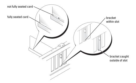
**4** Secure the card bracket with the screw you removed in step 2.
