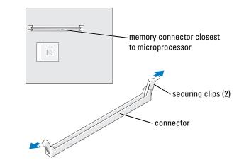
8 To insert a module, press out the securing clip at each end of the memory module connector.
