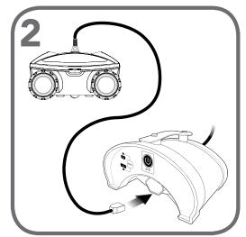
Straighten out the floating cable. Then lift the flap on the power supply. Plug in the cable.
