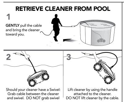
To avoid a possible electrical shock, do not use this product if the floating cable appears to be damaged.
