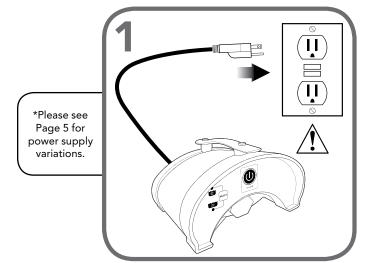
Plug power supply into a GFCI outlet (Ground Fault Circuit Interrupter) (Power Supply must be 12 ft. from the pool's edge)
