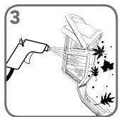
Use a hose to clean out the debris from the basket. Spray into the basket from the outside.
