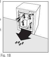
**IMPORTANT: Retain all shipping bolts, spacers and** grommets Reinstall to prevent damage if you transport machine in the future. Fig. 2
