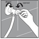
IMPORTANT: Do not over-tighten. Excessive force can damage the couplings. Tighten by hand; use a tool only in case of a leak.
