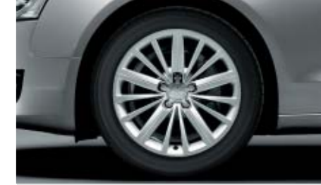
Cast aluminium winter wheels, 15-spoke star design, size 8.5 J x 18 with 245/40 R 18 tyres, permissible top speed 240 km/h, cannot be fitted with snow chains
