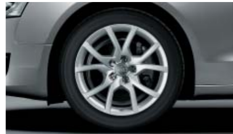
Cast aluminium wheels, 10-spoke V design, size 8.5 J x 18 with 245/40 R 18 tyres (only for 3.2 FSI and 3.0 TDI)
