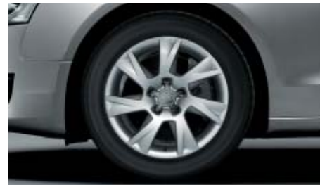
Cast aluminium wheels, 7-arm design, size 7.5 J x 17 with 225/50 R 17 tyres
