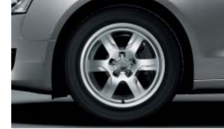
Lightweight forged aluminium winter wheels, 6-arm design 1 , size 7.5 J x 17 with 225/50 R 17 tyres, permissible top speed 210 km/h, can be fitted with snow chains
