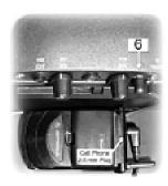
The ComSystem provides an input for cellular phone communication. Given the increased emphasis / local legislation requiring the use of cellular phone headsets while driving a car, as well as the proliferation of phone models and calling plans available, BMW is providing a simple connection to the ComSystem via the cellular phone headset 2.5 mm jack found on most phones. If your phone does not have a headset jack, consult your phone supplier for an accessory headset adapter.
