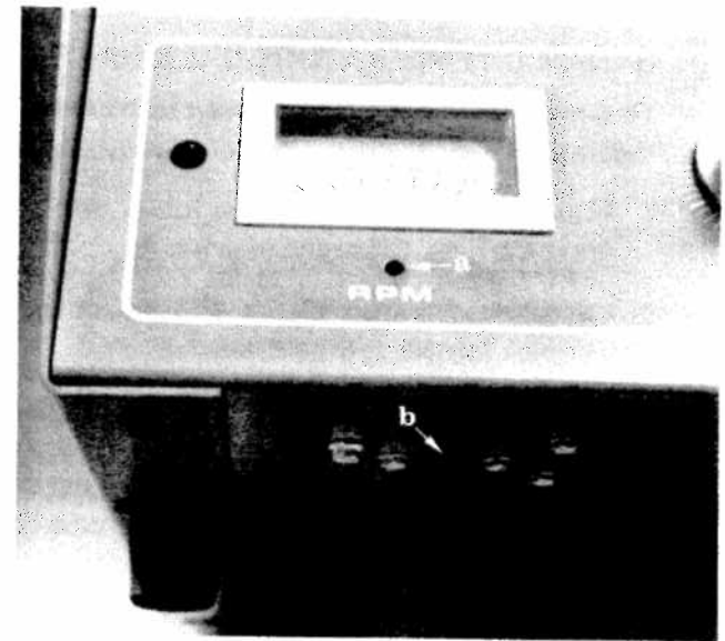
Figure 19. RPM Meter, Showing Zero Adjust ( a ) and Calibration ( b ) Hole
