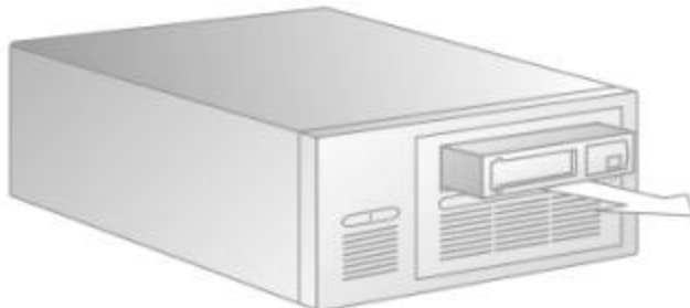
Figure 3-3: Unloading a DLTape Cartridge
