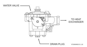
Fig. 1 - Water heater drain plug
