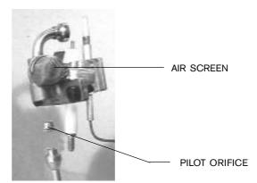
Fig. 11 - Pilot burner with air screen/ pilot orifice
