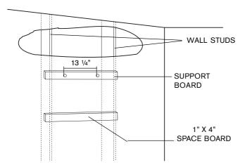
Fig. 2 - Mounting the Heater
