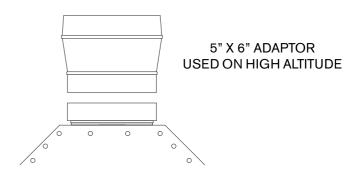
Fig. 4 - Vent Adaptor for High Altitude Installations
