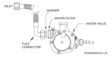
Fig. 6 - Water valve and water connector, top view
