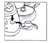
3. Place the protective cover (24) onto the chopping blade (23) and place into storage compartment. The highest part of the blade should be placed at the back of the compartment.
