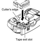
Make sure that the end of the tape feeds under the tape guides. Use only Brother M tapes with this machine.
