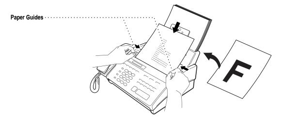
■ The automatic document feeder (ADF) can hold up to 10 pages, feeding each one individually through the fax machine. Use standard (17 lb–24 lb) paper when using the ADF; if you're using heavier paper, feed each sheet individually to prevent paper jams.
