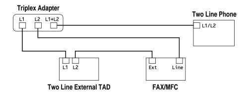
You can keep two-line telephones on other wall outlets as always. There are two ways to add a two-line telephone to the FAX/MFC's wall outlet. You can plug the telephone line cord from the two-line telephone into the L1+L2 jack of the triplex adapter. Or, you can plug the two-line telephone into the TEL jack of the two-line TAD.
