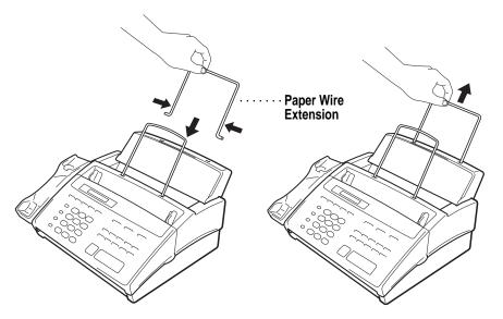
2 Insert the paper support into the openings as shown and then pull it out until you feel it click into place.
