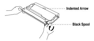
**5** Install the printing cartridge by inserting the indented  $\triangle$  first and placing the cartridge into its four holders.
