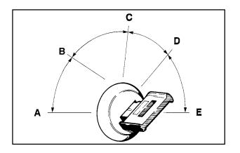
ACCESSORY (A): This position lets you use your electrical power accessories such as power windows, power sunroof (if equipped), radio and the windshield wipers. To use, push in the ignition key and turn it toward you. Your steering wheel will remain locked, just as it was before you inserted the key.
