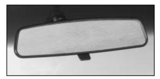
When you are sitting in a comfortable driving position, adjust the mirror so you can see clearly behind your vehicle. The day-night adjustment allows you to adjust the mirror to avoid glare from the headlamps behind you.
