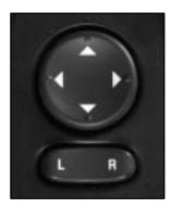
Your vehicle has a remote mirror control located on the driver's door armrest.
