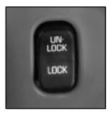
With power door locks, you can lock or unlock all the doors of your vehicle using the driver's or front passenger's door lock switch.
