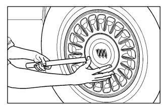
1. If your vehicle has an aluminum wheel with a center cover that hides the wheel nuts, remove the center cover by using the flat end of the wheel wrench to pry it off.
