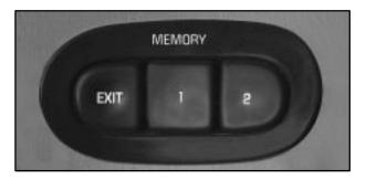
The controls for the memory seat and mirrors are located on the driver's door panel, and are used to program and recall previous settings that have been stored.
