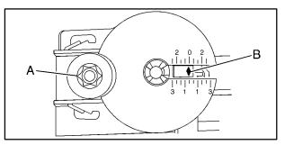
Once the horizontal aim is adjusted, then adjust the vertical aim.
