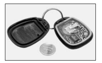
For battery replacement, use one Duracell<sup>®</sup> battery, type DL-2032, or a similar type.
