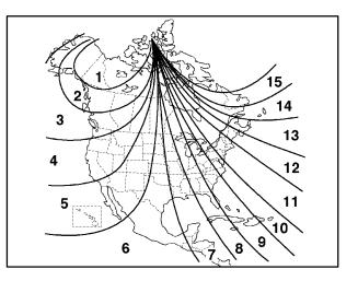
3. Press the COMPASS button on the bottom of the mirror until the new zone number appears in the display. After you stop pressing the button, the display will show a compass direction within a few seconds. (This is the automatic calibration mode. Drive in a circle to calibrate the mirror. See "Compass Calibration" explained previously.)
