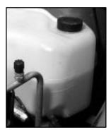
When the engine is cold, the coolant level should be at or above the FULL COLD mark (if the engine is hot, the coolant level should be at FULL HOT). If it isn't, you may have a leak in the radiator hoses, heater hoses, radiator, water pump or somewhere else in the cooling system.
