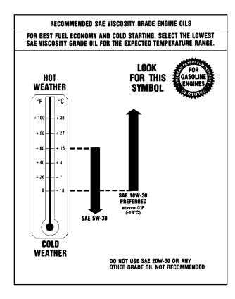
As shown in the chart, SAE 10W-30 is best for your vehicle. However, you can use SAE 5W-30 if it's going to be colder than 60°F (16°C) before your next oil change. When it's very cold, you should use SAE 5W-30. These numbers on an oil container show its viscosity, or thickness. Do not use other viscosity oils, such as SAE 20W-50.
