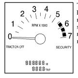
The tachometer tells you how fast the engine is running. It displays engine speed in thousands of revolutions per minute (rpm).
