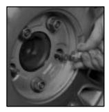
10. Replace the wheel nuts with the rounded end of the nuts toward the wheel.
