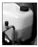
The vehicle must be on a level surface. When your engine is cold, the coolant level should be at FULL COLD or a little higher. When your engine is warm, the level should be up to FULL HOT or a little higher.
