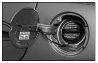
The cap is behind a hinged door located on the driver's side of your vehicle.
