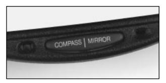
The right side of the switch located at the bottom of the mirror turns the electrochromic mirror on and off. To turn on the automatic dimming feature, press MIRROR. To turn off automatic dimming, press MIRROR again. The green indicator light will be illuminated when this feature is active.
