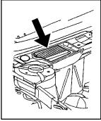
The particle filter is under a removeable panel located at the base of the windshield on the passenger's side.
