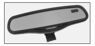
When set in the MIRROR position, this mirror automatically changes to reduce glare from headlamps behind you. A time delay feature prevents rapid changing from the day to night positions while driving under lights and through traffic.
