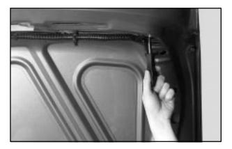
1. Loosen and remove the seven fasteners that hold the assembly in place. The assembly for both sides is one piece. The entire piece must be removed to replace any bulbs.
