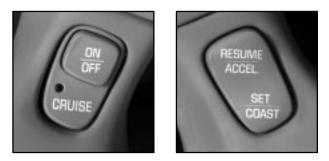
The controls to operate the cruise control are located on the steering wheel.
