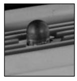
Your Twilight Sentinel and DRL work with the light sensor located on top of the instrument panel.
