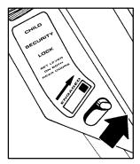
Your vehicle is equipped with rear door security locks that help prevent passengers from opening the rear doors of your vehicle from the inside.
