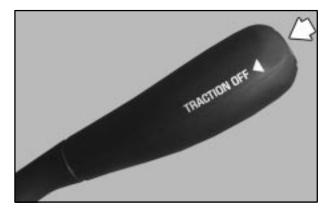
To turn the system off, press the TRACTION OFF button located at the end of the shift lever on the right side of the steering wheel.
