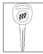
There is a master key that works in all of the lock cylinders (doors, trunk, ignition, and glove box). Both the master and VALET key have a transponder embedded into the key for security and vehicle theft deterrence. The keys also come with a bar code tag. Keep the bar code tag in a safe place. If you lose your key, you will be able to have a new one made using the bar code tag. The replacement key must have a vehicle theft deterrent system transponder embedded in it.
