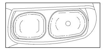
2. Measure the distance from the ground to the aim dot on each lamp; if left low beam, subtract two inches. Record this distance. 3. At the wall or other flat surface, measure from the floor to the recorded distance and draw a horizontal line the width of the vehicle.
