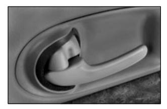
To unlock the door from the inside, move the manual door lock control located above the door handle rearward. To lock the door, move the manual door lock control forward.
