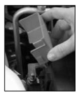
Start by lifting and moving the red positive (+) remote terminal cover away from the relay center.
