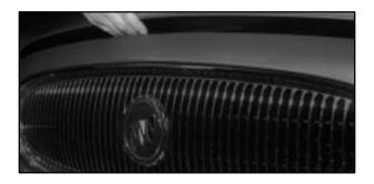
Then go to the front of the vehicle and pull up on the secondary hood release. The hood latch is located under the hood, near the center, and at the front edge of the grille. Lift up on the latch as you lift up on the hood.
