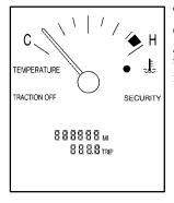
This gage shows the engine coolant temperature. If the gage pointer moves into the red area, your engine is too hot!
