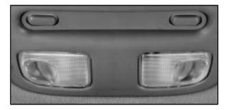
Front seat reading lamps are turned on or off by pressing one of the lamps buttons.
