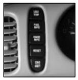
The following buttons are on the DIC control panel which is located to the left of the steering column:
