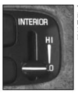
The brightness of the instrument panel lights can be adjusted by moving the INTERIOR lever between LO and HI.
