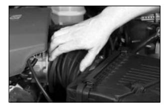
2. Remove the air intake hose that is snapped over the throttle body by pulling the hose upward and away from the throttle body which is located near the top of the engine.
