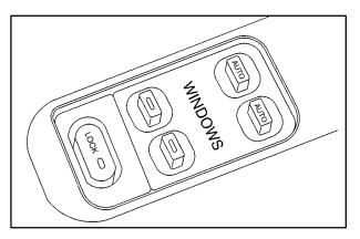
The power window controls located on the driver's armrest operate each of the windows while the ignition is on or while retained accessory power is active. In addition, each passenger door has a control for its own window.
