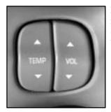
Press the TEMP up arrow to increase the temperature and the TEMP down arrow to decrease the temperature.
