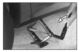
3. Turn the wheel wrench counterclockwise to lower the jack head until it fits under the vehicle.
