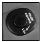
The TRUNK PUSH OPEN release button is on the driver's door trim map pocket. Push this button to open the trunk. The transaxle must be in PARK (P) or NEUTRAL (N) for the remote trunk release button to work.
