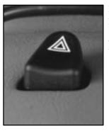
Press this button to make your front and rear turn signal lamps flash on and off. It is located on top of the steering column.
