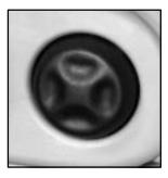
The lumbar control is located on the outboard side of each front seat. Use the power seat control first to get the proper position. Then continue with the lumbar adjustment.
