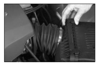
The air cleaner and filter are located on the driver's side of the engine compartment.
