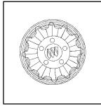
2. If your vehicle has this aluminum wheel, you may have plastic wheel nut caps. Use the wheel nut wrench to remove the wheel nut caps and to loosen the wheel nuts.
