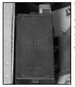
The rear BEC is located beneath the rear seat on the driver's side. The rear seat cushion must be removed to access the BEC. See "Removing the Rear Seat Cushion" in the Index.
