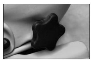
The knob that controls this feature is located on the outer edge of the seat. Turn the knob towards the front of the vehicle to increase lumbar support. Turn the knob towards the rear of the vehicle to decrease lumbar support.
