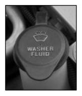
If your vehicle is not equipped with a DIC, a washer dip tube has been provided to check fluid level. Place fingers over the holes on the dip tube handle and pull the tube out of the bottle. If there is no fluid in the tube, windshield washer fluid needs to be added.
