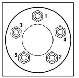
Tighten the wheel nuts firmly in a crisscross sequence.
