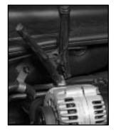
It goes to a heavy, unpainted metal part on the engine of the vehicle with the dead battery.
