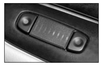
If your vehicle is equipped with the Dual Automatic Comfortemp system, the front seat passenger can control the air temperature in their seating area. The control is located on the passenger's door armrest.
