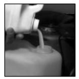
4. Then fill the coolant recovery tank to the FULL COLD mark.
