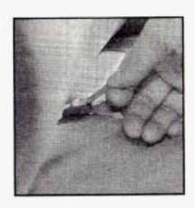
Reach over the second row seat and pull up on the strap loop. Then pull the seat cushion up and push it forward.
