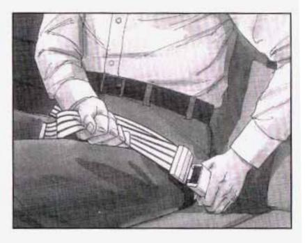
To make the belt shorter, pull its free end as shown until the belt is snug. Buckle, position and release it the same way as the lap part of a lap-shoulder belt. If the belt isn't long enough, see Safety Belt Extender on page 1-47.
