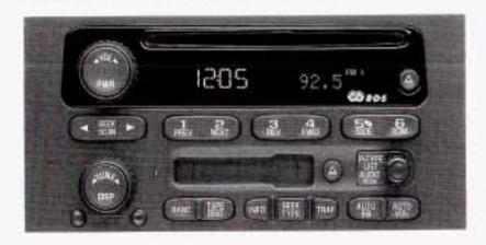
Radio Data System (RDS): Your audio system is equipped with a Radio Data System (RDS). RDS features are available for use only on FM stations that broadcast RDS information. With RDS, your radio can do the following:
