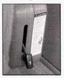
To return the seatback to an upright position, pull up on the release lever labeled 1 and then pull up on the seatback until it locks into the upright position.
