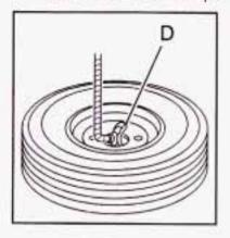
Tilt the retainer (D) downward and through the wheel opening. Make sure the retainer is fully seated across the underside of the wheel.
