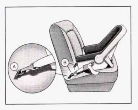
With this system, use the LATCH system instead of the vehicle's safety belts to secure a child restraint.
