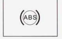
With the anti-lock brake system, this light will come on when you start your engine and may stay on for several seconds.
