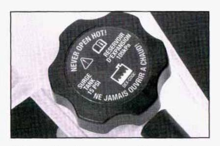
Then replace the pressure cap. Be sure the pressure cap is hand-tight and fully seated.
