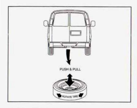
Make sure the tire is stored securely. Push, pull, and then try to rotate or turn the tire. If the tire moves, use the wheel wrench to tighten the cable. Reinstall the spare tire lock (if equipped).
