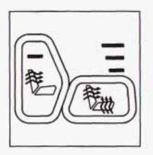
The buttons used to control this feature are located on the front doors. The engine must be running for the heated seat feature to work.
