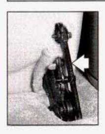
While holding the seat forward, pull the prop rod out from the retainer clips. Flip the prop rod (arrow) down until it latches into place.
