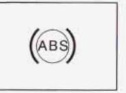
If there's a problem with the anti-lock brake system, this warning light will stay on. See Anti-Lock Brake System Warning Light on page 3-38.
