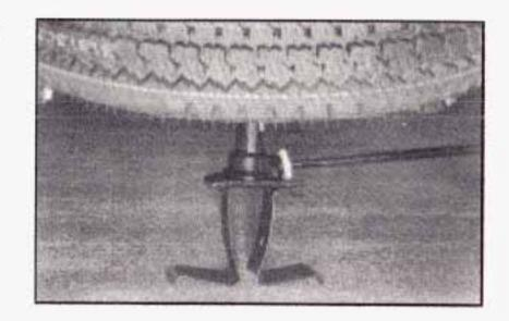
Place the bottom edge of the jack on the wheel blocks, separating them so that the jack is balanced securely.
