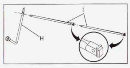
Assemble the wheel wrench (H) and the two jack handle extensions (I) as shown.
