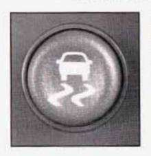
Stabilitrak® and part of the traction control system can be turned off or back on by pressing the Stabilitrak® button located on the instrument panel.
