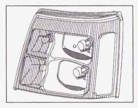
Measure the distance from the ground to the aim dot on each low beam lamp. Record this distance.  At the wall or other flat surface, measure from the ground upward the recorded distance from Step 2 and draw or tape a horizontal line the width of the vehicle.
