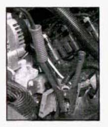
The remote positive (+) terminal is located under a red plastic cover near the engine accessory drive bracket. To access the remote positive (+) terminal, open the red plastic cover.
