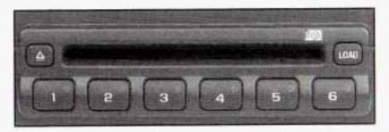
The compact disc changer plays up to six standard size CDs continuously. Individual CDs may be loaded or ejected into or from any position.
