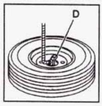
Tilt the retainer at the end of the cable and pull it through the wheel opening. Pull the tire out from under the vehicle.  If the cable is hanging under the vehicle, turn the wheel wrench in the hoist shaft hole in the bumper clockwise to raise the cable back up.
