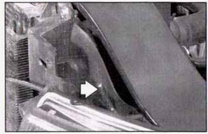
Remove the horizontal pin from the headlamp assembly by lifting the end of the pin upward until it unsnaps and then pulling it toward the center of the vehicle.
