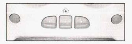
HomeLink<sup>®</sup>, a combined universal transmitter and receiver, provides a way to replace up to three hand-held transmitters used to activate devices such as gate operators, garage door openers, entry door locks, security systems and home lighting. Additional HomeLink<sup>®</sup> information can be found on the internet at www.homelink.com or by calling 1-800-355-3515.
