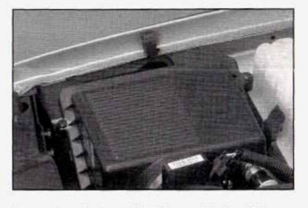
Your engine air cleaner/filter is located in the air filter housing near the front corner of the engine compartment on the passenger's side of the vehicle. See *Engine Compartment Overview on page 5-12* for more information on location.
