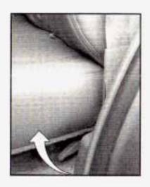
Pull the seatback release lever upward and pull the seatback up and fold it down until it is flat. Escalade lever shown, Escalade ESV lever similar.
