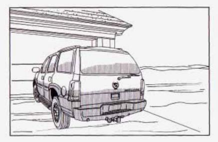
Turn on the low-beam headlamps and place a piece of cardboard or equivalent in front of the headlamp not being aimed. This should allow only the beam of light from the headlamp being aimed to be seen on the flat surface.
