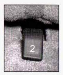
To unlatch the rear of the seat from the floor, pull up on the release lever labeled 2 at the rear of the seat and lift the rear of the seat up from the floor.
