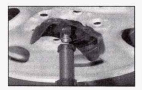
Attach the jack handle, extension, and wheel wrench to the jack and place it (with the wheel blocks) under the vehicle towards the front of the rear bumper. Position the center lift point of the jack under the center of the spare tire.
