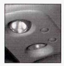
If your vehicle has reading lamps, press the button located next to the lamp to turn it on. The lamps can be adjusted to point in the direction you want.
