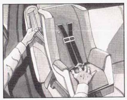
To tighten the belt, feed the shoulder belt back into the retractor while you push down on the child restraint. If you are using a forward-facing child restraint, you may find it helpful to use your knee to push down on the child restraint as you tighten the belt. You should not be able to pull more of the belt from the retractor once the lock has been set.
