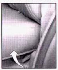
Pull up the lever located under the seat cushion. Escalade lever shown, Escalade ESV lever similar.
