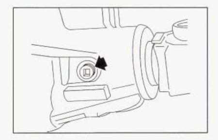
To get an accurate reading, the vehicle should be on a level surface. The proper level is from 5/8 inch to 1 5/8 inch (15 mm to 40 mm) below the bottom of the filler plug hole. Add only enough fluid to reach the proper level.
