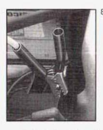
Now connect the black negative (-) cable to the negative (-) terminal of the good battery. Use a remote negative (-) terminal if the vehicle has one. Your vehicle's remote negative (-) terminal is marked GND.
