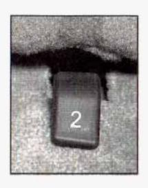
To unlatch the rear of the seat from the floor, pull up on the release lever labeled 2, at the rear of the seat, and lift the rear of the seat up from the floor.
