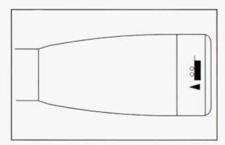
Your vehicle is equipped with a tow/haul mode. The button for this feature is located on the end of the column shift lever. You can use this feature to assist when towing or hauling a heavy load. See "Tow/Haul Mode" under Towing a Trailer on page 4-50 for more information.
