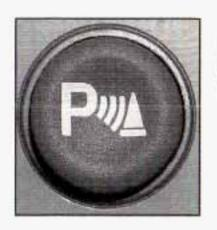
URPA can be disabled by pressing the URPA on/off button located near the climate control system and radio
