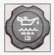
The engine oil fill cap is located on the valve cover on the passenger's side of the vehicle. See Engine Compartment Overview on page 5-12 for further location information.
