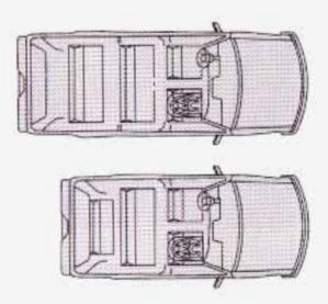
Your vehicle has a right front passenger air bag. A rear seat is a safer place to secure a forward-facing child restraint. Unless your vehicle has the passenger sensing system, never put a rear-facing child restraint in this seat. Here's why:
