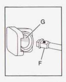
Insert the hoist end (open end) (F) of the extension through the hole (G) in the rear bumper.
