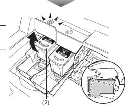
6 Lift the Scanning Unit (Printer Cover) slightly to set the Scanning Unit Support back to its original position, and then gently close the Scanning Unit (Printer Cover).
