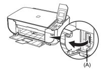
Insert one and only one memory card into the Card Slot.
