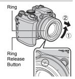
Align the ● mark on the conversion lens adapter with the ● mark on the camera, and turn the adapter in the direction of the arrows until locked (as far as the ▲ mark on the camera).
