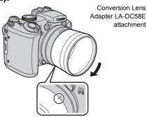
To remove the conversion lens adapter (lens hood or conversion lens), turn the adapter in the opposite direction with holding down the ring release button. 4
