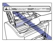
Keep your hands or clothing away from the roller in the output area after removing jammed paper completely. Even if the printer is not printing, sudden rotation of the roller may catch your hands or clothing, resulting in personal injury.
