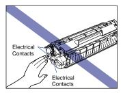
• Whenever you are handling the toner cartridge, hold it as shown in the diagram, and keep the surface marked with the arrow facing up. Do not stand it on its end, or turn it upside down.
