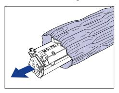
8 Align the protrusions on the left and right ends of the toner cartridge with the toner cartridge guides in the main printer, and push the cartridge all the way to the back ①, then pull it down towards you 2.
