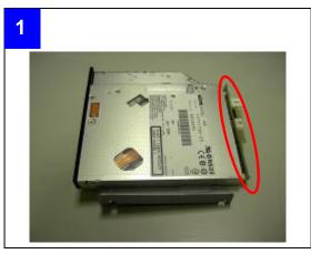
Assemble the adapter board with attached screws onto Slim ODD
