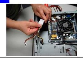
■ Use power split cable in accessory pack for conversion of DC harness, small 4P is connected to the Slim **ODD** adaptor board
