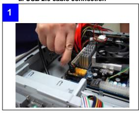
■ Front USB cable should be connected to on-board USB header properly depends on different M/B.
