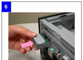
■ Install the assembled Card Reader back to the chassis with screw
