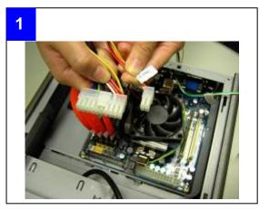
■ The DC harness comes with 20+4 pin as main connection for different M/B requirement.
