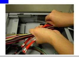
■ Due to limited space inside the chassis, make sure all cable are connected properly and use the cable tie through the bridge land on side wall
