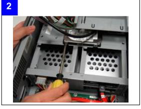
■ Place 2.5" HDD underneath the Slim ODD
