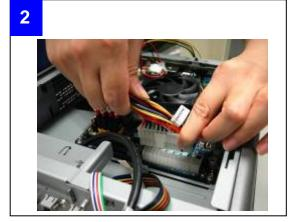
■ Install and secure the DC harness cable to the M/B properly
