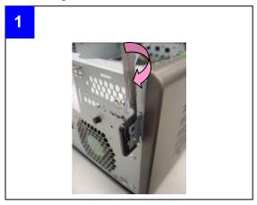
■ Remove the cap on slot holder
