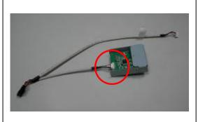
■ Connect the short end of USB split cable to Card Reader
