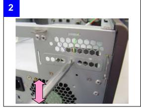
■ Detach the low profile slot bracket from rear window
