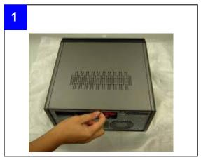
■ Release the side panel thumb screw on the rear
