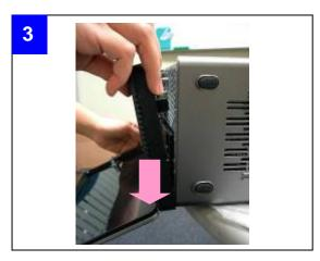
■ Angle the latch until it is 15 degree away from the chassis
