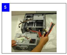
■ Finish detaching the M/B cage and make sure all the connection on backplane and PDB are still tight before assembly back the M/B cage
