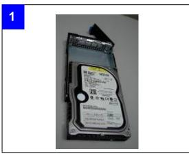
■ Remove the HDD Carrier from the chassis and place the SATA-II HDD into it.
