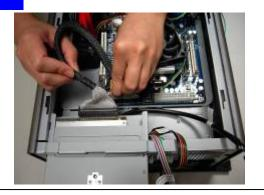
■ Use either standard IDE / SATA cable from 3<sup>rd</sup> party M/B, or use optional cable from Chenbro to connect to the Slim ODD adaptor board
