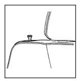
5. Pull up on the knob located on the top of the seatback on the outboard side to release the seatback. With your other hand, pull the seatback forward.
