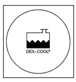
The coolant recovery tank cap has this symbol on it. The tank is located in the engine compartment toward the front of the engine on the passenger's side of the vehicle.
