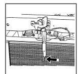
2. Then go to the front of the vehicle and push the secondary hood release lever to the left. It is located under the front center of the grille.
