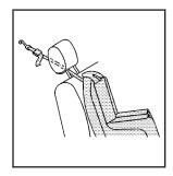
If the position you are using has a fixed or adjustable head restraint and you are using a single tether, route the tether under the head restraint and in between the head restraint posts.
