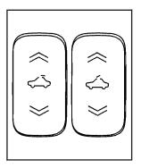
The switches that operate the sunroof are located in the headliner.
