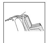
If the position you are using does not have a head restraint and you are using a dual tether, route the tether over the seatback.
