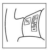
The cruise control buttons are located on the left side of the steering wheel. (S) (**On/Off):** Press this button to turn the cruise control system on and off. The indicator light on the button will be on when the cruise control is on and go off when the cruise control is turned off.
