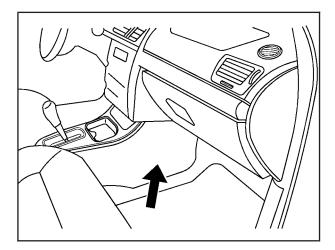
The floor console fuse block is located on the passenger's side of the floor console behind the forward panel. The panel has four clips, one in each corner. Pull the panel to disconnect the four clips, and access the fuses. Use the fuse puller to remove fuses.
