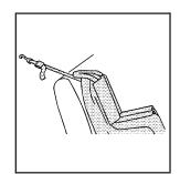
If the position you are using does not have a head restraint and you are using a single tether, route the tether over the seatback.
