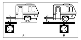
If you are using a weight-carrying hitch, the trailer tongue (A) should weigh 10 to 15 percent of the total loaded trailer weight (B).
