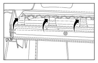
3. Pull each of the three tabs of the filter access door down and open the access door downward.
