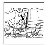
The remote positive terminal is located under a red tethered cap on the engine compartment fuse block. Remove the cap to access the terminal.
