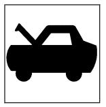
1. Pull the interior hood release lever with this symbol on it. It is located to the left of the instrument panel on the driver's side of the vehicle.
