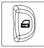
The power door lock switches are located on the driver's and front passenger's door next to the door handle.
