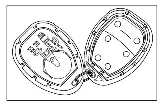
To replace the battery in the remote keyless entry transmitter do the following:
