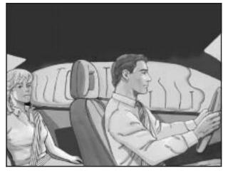
If your vehicle has a roof-mounted side impact airbag for the driver and the person seated directly behind the driver, it is located in the ceiling above the side windows.
