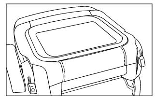
4. Continue to fold the seat forward until it locks in the folded position. Pull up on the seatback to be sure it is locked.
