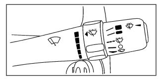
Use this lever, located on the right side of the steering wheel, to operate the windshield wipers.
