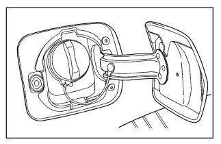
The tethered fuel cap is located behind a hinged fuel door on the passenger's side of the vehicle.
