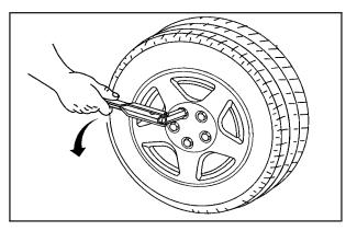
1. Using the wheel wrench, loosen all the wheel nuts. Do not remove them yet.
