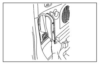
2. Remove the cover in the rear cargo area of the vehicle to access the bulbs.
