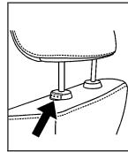
Pull the head restraint up to raise it. To lower the head restraint, press the button, located on the top of the seatback, and push the restraint down. Only the front head restraints are adjustable.
