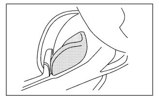
To tilt the wheel, pull the lever down. Then, move the wheel to a comfortable position and raise the lever to lock the wheel in place.
