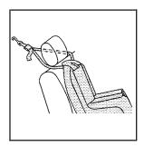
If the position you are using has a fixed or adjustable head restraint and you are using a dual tether, route the tether around the head restraint.
