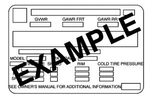
A vehicle specific Certification/Tire label is found on the rear edge of the driver's door.
