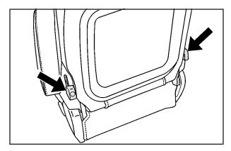
Use one of two levers to fold the seat flat. The levers are located on the rear of the seat near the bottom of either side of the seat. Pull up on either lever and fold the seat forward until the seatback disengages. This can most easily be down from the rear seats.
