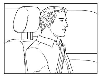
Adjust the head restraint so that the top of the restraint is at the same height as the occupant's head. This position reduces the chance of a neck injury in a crash.
