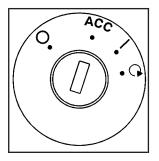
*Notice:* Using a tool to force the key from the ignition switch could cause damage or break the key. Use the correct key and turn the key only with your hand. Make sure the key is all the way in. If it is, turn the steering wheel left and right while you turn the key hard. If none of this works, then your vehicle needs service.
