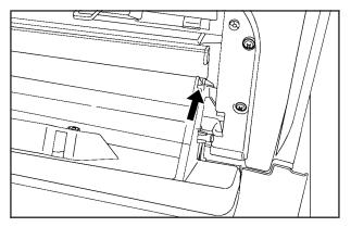
2. Release the glove box stops by pushing them both outward to let the glove box drop open completely.
