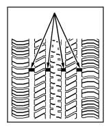
One way to tell when it is time for new tires is to check the treadwear indicators, which will appear when your tires have only 1/16 inch (1.6 mm) or less of tread remaining.
