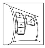
Radio controls are located on the right side of the steering wheel. If your vehicle has this feature, some audio controls can be adjusted at this location. They include the following: + - (Volume): Press the plus or minus button to increase or to decrease the volume.
