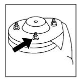
The remote negative (–) ground terminal, marked GND (–), is located at the front of the engine compartment on the driver's side of the vehicle.
