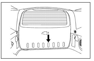
1. Remove the trim plug, located on the inside of the liftgate near the center.
