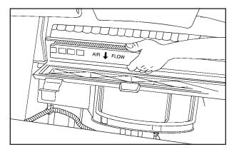
4. Pull the filter out, keeping it face up so as not to drop any dust into the passenger compartment upon removal.
