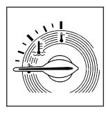
Your vehicle has an engine coolant temperature gage. With the ignition turned to RUN, this gage shows the engine coolant temperature.
