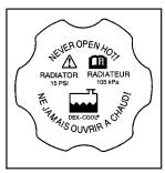
1. You can remove the pressure cap when the cooling system, including the pressure cap and upper radiator hose, is no longer hot. Turn the pressure cap slowly counterclockwise.
