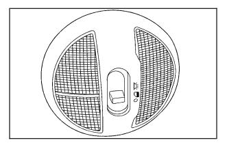
○ (Off): Move the lever to this position to turn the lamp off, even when a door is opened.
