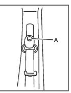
To move it down, press the release button (A) and move the height adjuster to the desired position. You can move the height adjuster up just by pushing up on the shoulder belt guide.
