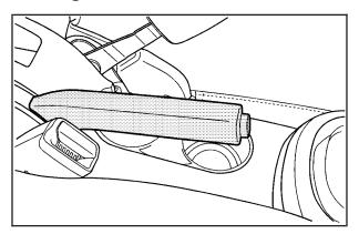
The parking brake lever is located between the front seats.
