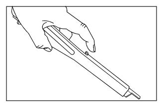
Press the button and then pull on the end of the wheel wrench to extend the handle.
