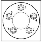
11. Tighten the wheel nuts firmly in a crisscross sequence, as shown.
