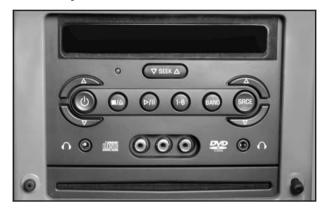
( (Power): Press this button to turn the RSE system on and off.
