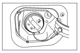
The fuel cap is located behind a hinged door on the passenger's side of your vehicle. To open the door, insert your finger into the finger depression next to the fuel door.
