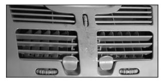
Use the horizontal thumbwheels on the air outlets, located in the center and on the sides of the instrument panel, to change the direction of the airflow. Airflow can be shut off at the center upper outlet by turning the vertical thumbwheel. The other outlets can be shut off by closing the outlet vanes.
