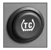
To turn the system on or off, press the ETS button on the center console under the climate control system.
