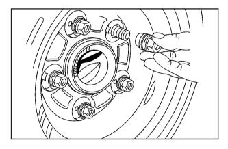
Install the compact spare tire. Put the wheel nuts back on with the cone end of the nuts toward the wheel. Tighten each nut by hand or with the wrench until the wheel is held against the hub.
