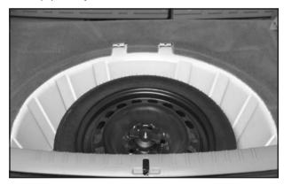
For the sedan model, lift the handle on the spare tire cover. The handle may hook on the trunk front edge weatherstrip to hold the cover out of the way. For the MAXX model, lift the handle to release the latch on the spare tire cover.
