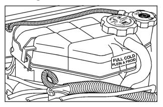
The engine coolant surge tank is located in the rear of the engine compartment. See *Engine Compartment Overview on page 5-14* for more information on location.
