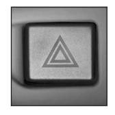
The hazard warning flasher is located near the center of the instrument panel.
