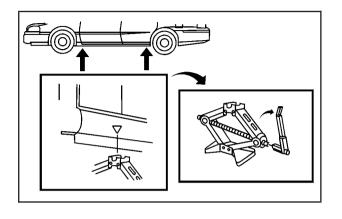
4. Position the lift head at the jack location nearest the flat tire. Make sure all of the jack lift head is touching the jacking flange under the body. Do not place the jack under a body panel. The lower body panel has an arrow to aid in location the jacking location. Put the compact spare tire near you.
