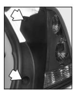
2. Unscrew the two fasteners located on the inside of the trunk at the rear of the vehicle.
