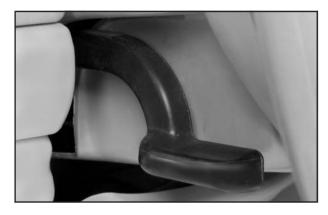
To tilt and telescope the wheel, pull down the lever. Then move the wheel to a comfortable position, pull up the lever to lock the wheel in place. The wheel can be adjusted up and down as well as forward and backward.
