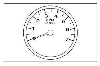
The tachometer shows your engine speed in revolutions per minute (rpm).
