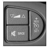
$\nabla$  **SEEK**  $\triangle$ : Press the up or the down arrow to go to the next or to the previous radio station.
