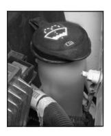
The windshield washer fluid reservoir is located on the driver's side of the engine compartment. See Engine Compartment Overview on page 5-14 for reservoir location.
