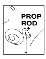
Release the hood prop rod from its retainer and put the hood prop into the slot marked with an arrow. Before closing the hood, be sure all the filler caps are on properly. Lift the hood to relieve pressure on the hood prop. Then let the hood drop from about 8 to 12 inches (20 to 30 cm) above the vehicle to latch fully. Do not drop the hood from full prop-rod height. Check to make sure the hood is closed and repeat the procedure if necessary.
