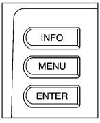
The buttons used to activate the DIC are located on the left side of the vehicle's audio controls.
