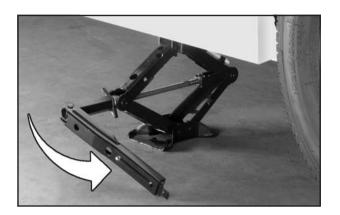
Lower the vehicle by turning the wrench counterclockwise. Lower the jack completely.
