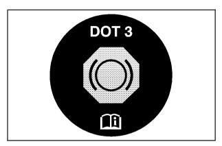
Your brake master cylinder reservoir is filled with DOT-3 brake fluid. See *Engine Compartment Overview* on page 5-14 for the location of the reservoir.
