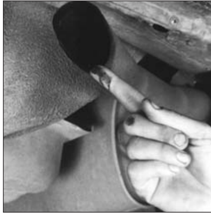
7.5 Check the tailpipe - black, sooty deposits at the end of the exhaust pipe may be an indication that the carburetor needs adjustment or the engine is in need of a tune-up
