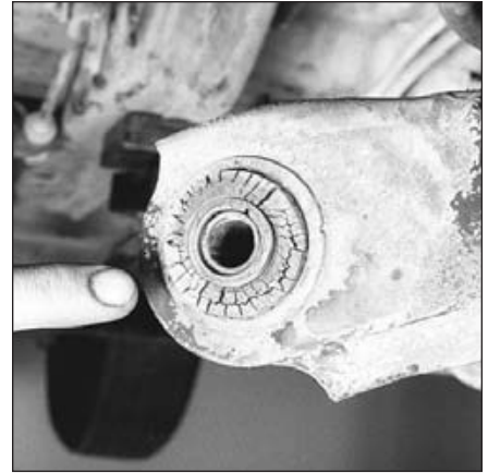
8.6a Cracked rubber bushings in the steering and suspension systems should be replaced
