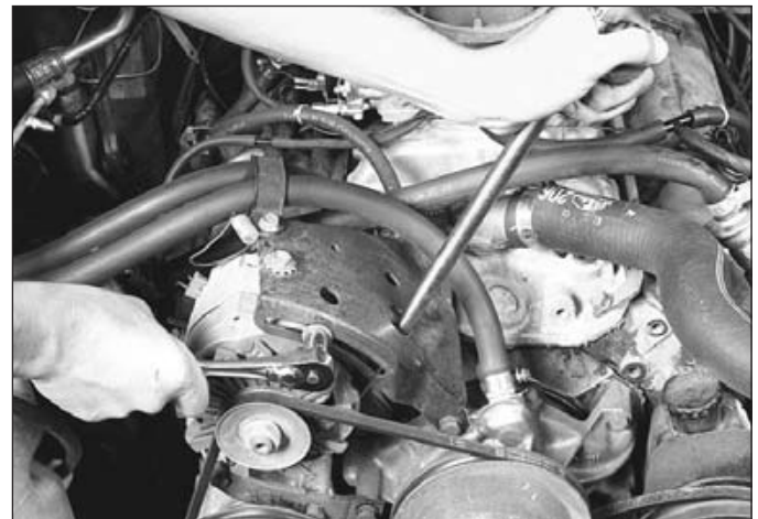
9.8 Adjust the belt tension by gently prying on the component as the adjustment bolt is tightened
