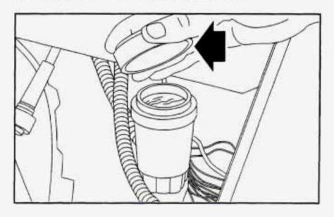
Refer to the Maintenance Schedule, Owner Checks and Services, to determine how often you should check the fluid level in your clutch master cylinder reservoir and for the proper fluid. See "Owner Checks and Services" and "Recommended Fluids and Lubricants" in the Index.
