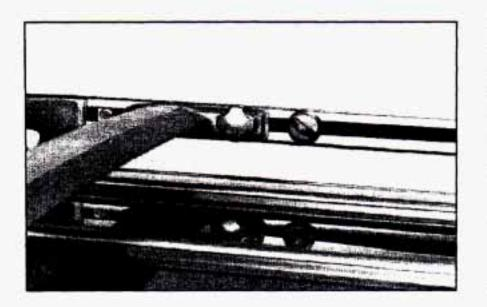
Remove the center rubber strips in the crossrails and attach the GM accessory rack to the nut plates provided through the center slots (four per crossrail).
