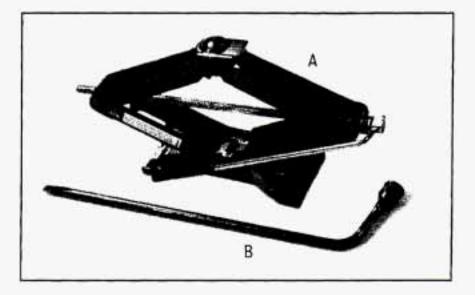
The tools you'll be using include the jack (A) and wheel wrench (B). Your vehicle may also have an optional hub cap removal tool.
