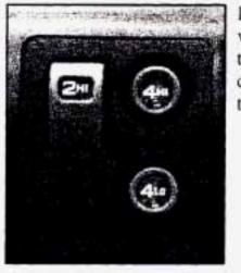
If your four-wheel-drive vehicle has the electronic transfer case, the transfer case switches are above the radio controls.
