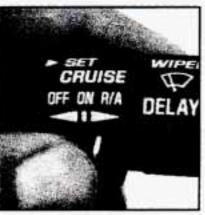
Once you're going about 25 mph (40 km/h) or more, you can move the cruise control switch from ON to R/A for about a half a second.
