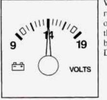
When your engine is not running, but the ignition is on (in the RUN position). this gage shows your battery's state of charge in DC volts.
