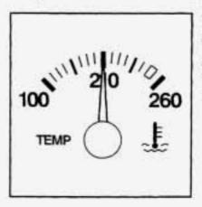
This gage shows the engine coolant temperature. If the gage pointer moves into the red area, your engine is too hot!
