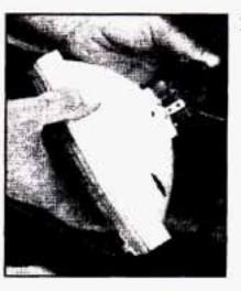
Pull the headlamp out and remove the retainer.
