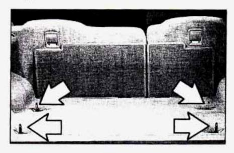
There are four cargo tie downs in the rear that allow you to strap cargo in and keep it from moving inside the vehicle. Luggage Carrier (If Equipped)
