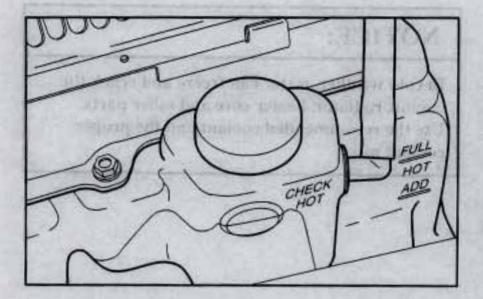
The coolant level should be at the ADD mark.
