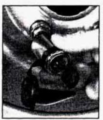
Insert the key and pull the lock case straight off. It is not necessary to turn the key.
