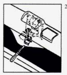
Use a thin screwdriver to reach through the access holes in both the trim panel and the hardware cover.
