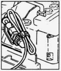
In very cold weather, 0°F (-18°C) or colder, the engine coolant heater can help.
