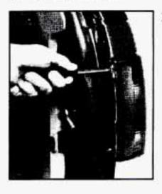
Remove the two screws from the lamp assembly.
