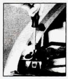
Remove the black protective caps from the removal pins at the top of the radiator support. Use a hex socket to unscrew the pins.
