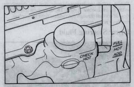
When your engine is cold, the coolant level should be at ADD, or a little higher. When your engine is warm, the level should be up to FULL HOT, or a little higher.
