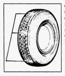
One way to tell when it's time for new tires is to check the treadwear indicators, which will appear when your tires have only 1/16 inch (1.6 mm) or less of tread remaining.
