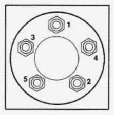
Use the wrench to tighten the wheel nuts firmly in a crisscross sequence as shown.
