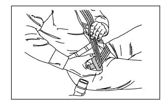
If the belt stops before it reaches the buckle, tilt the latch plate and keep pulling until it can be buckled.
