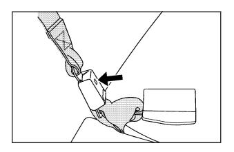
Detach the center safety belt from the mini buckle by inserting the ignition key into the slot in the mini buckle, pressing the release button, and allowing the belt to retract.
