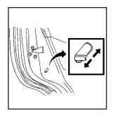
Your vehicle has rear door security locks on each rear door that prevent passengers from opening the rear doors from the inside.
