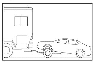
The vehicle can be towed from the front using a dolly. To tow the vehicle using a dolly, follow these steps:
