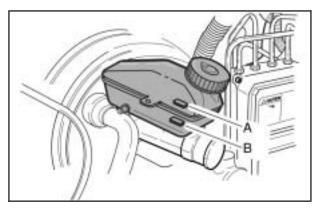
To check the fluid level, look on the side of the reservoir. If the fluid reaches the MAX (A) mark on the reservoir, the fluid level is correct. If the fluid does not reach the MIN (B) mark on the reservoir, then fluid needs to be added.
