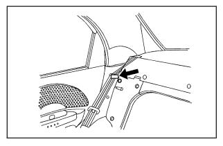
4. Hook the safety belts in the outboard seating positions into the retaining clips.
