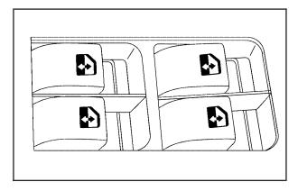
If your vehicle has power windows, the switches are located on the driver's door. In addition, each passenger door has a switch for its own window.
