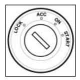
The ignition switch has four different positions.
