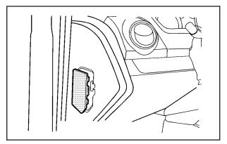
To access the fuses, open the fuse panel door by pulling the door out.
