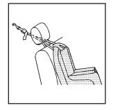
If the position you are using has a headrest or head restraint and you are using a dual tether, route the tether under the headrest or head restraint and in between the headrest or head restraint posts.
