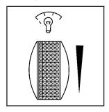
The thumbwheel for this feature is located on the instrument panel to the left of the steering column. Turn the thumbwheel to brighten or dim the lights.
