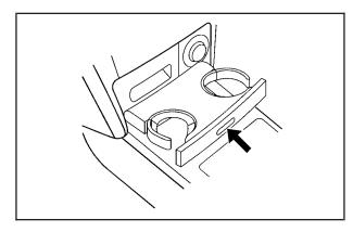
Two cupholders are located in the center instrument panel, below the climate control system. To use the cupholder, push in on the cover, then pull it out. After use, push in the cupholder until it latches.
