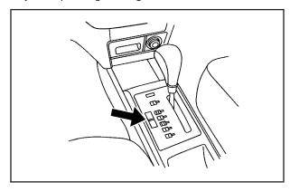
Press the HOLD button on the shift lever console to turn on hold mode. Press the button again to turn off hold mode, and return to normal automatic transmission operation. The HOLD light will light up on the instrument panel cluster. See *Hold Mode Light on page 3-30*.
