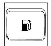
To open the fuel filler door, pull up on the release lever with this symbol on it. It is located on the floor on the outboard side of the driver seat.
