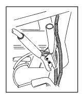
negative (–) terminal of the good battery. Use a remote negative (–) terminal if the vehicle has one. Do not let the other end touch anything until the next step. The other end of the negative (–) cable does not go to the dead battery. It goes to a heavy, unpainted metal engine part or to a remote negative (–) terminal on the vehicle with the dead battery.
