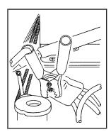
Do not let the other end touch metal. Connect it to the positive (+) terminal of the good battery. Use a remote positive (+) terminal if the vehicle has one.
