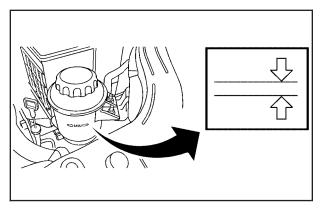
The level should be between the MIN (B) and MAX (A) marks on the reservoir. If the level drops below the MIN (B) mark, add power steering fluid. Do not overfill the reservoir and remember to replace the cap tightly when you are finished and clean up any spilled fluid.
