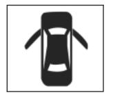
The door ajar light comes on and stays on until all doors, trunk and liftgate are closed and completely latched.
