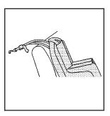
If the position you are using does not have a headrest or head restraint and you are using a dual tether, route the tether over the seatback.
