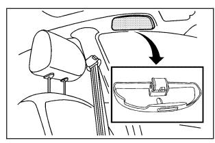
For vehicles with this feature, the sunglasses storage compartment is located above the driver's door. To open, pull down and hold the upper part of the cover. Release the cover and the compartment will automatically close.
