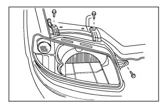
Reinstall the headlamp assembly using the three bolts.
