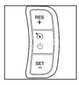
The cruise control buttons are located on the right side of the steering wheel.
