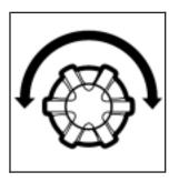
Turn the knob located on the outboard side of the seat cushion to adjust the height of the driver seat cushion.
