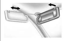
Pull the sun visor down to block glare. Detach the sun visor from the center mount to pivot to the side window, or to extend along the rod, if available
