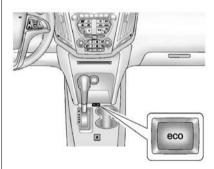
Press the "eco" (economy) button by the shift lever to turn this feature on or off. The "eco" light in the instrument cluster will come on when engaged, and a Driver Information Center (DIC) message "ECO MODE ON" displays. See Fuel Economy Mode on page 9-32.
