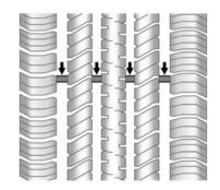
Treadwear indicators are one way to tell when it is time for new tires. Treadwear indicators appear when the tires have only 1.6 mm (1/16 in) or less of tread remaining. See *Tire Inspection on page 10-56* and *Tire Rotation on page 10-56* for more information.
