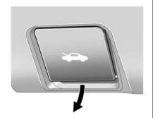
Pull the release handle located below the instrument panel to the left of the steering wheel.
