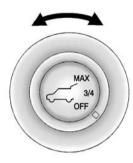
Choose the power liftgate mode by turning the dial on the switch until the indicator lines up with the desired position. The vehicle must be in P (Park).
