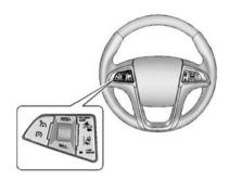
To turn LDW on and off, press the LANE DEPART control on the steering wheel. The control indicator will light when LDW is on.
