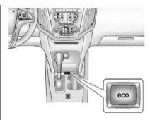
Press the "eco" (economy) button by the shift lever to turn this feature on or off. The "eco" light in the instrument cluster will come on when engaged. See Fuel Economy Light on page 5-22. A Driver Information Center (DIC) message "ECO MODE ON" is also displayed. See Fuel System Messages on page 5-30 for more information.
