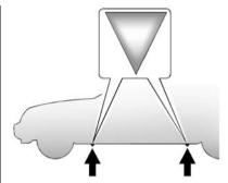
4. Position the jack lift head at the jack location nearest the flat tire. The location is indicated by a mark on the bottom edge of the front and rear door plastic molding. The jack must not be used in any other position.
