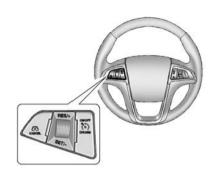
**ON/OFF**  $\mathfrak{S}$  **CRUISE**: Press to turn the cruise control system on and off.
