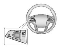
**ON/OFF** CRUISE: Press to turn the cruise control system on and off.
