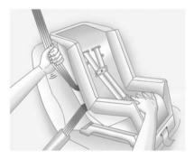
6. To tighten the belt, push down on the child restraint, pull the shoulder portion of the belt to tighten the lap portion of the belt, and feed the shoulder belt back into the retractor. When installing a forward-facing child restraint, it may be helpful to use your knee to push down on the child restraint as you tighten the belt. Try to pull the belt out of the retractor to make sure the retractor is locked. If the retractor is not locked, repeat Steps 5 and 6.
