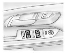
The power windows work when the ignition is in ON/RUN or ACC/ACCESSORY, or in Retained Accessory Power (RAP). See Retained Accessory Power (RAP) on page 9-25.
