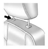
The height of the head restraint can be adjusted. Pull the head restraint up to raise it. Try to move the head restraint to make sure that it is locked in place.
