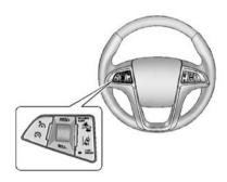
The Collision Alert control is on the steering wheel. Press COLLISION ALERT to set the alert timing to far, medium, near or off. The first button press shows the current control setting on the DIC. Additional button presses will change this setting. The chosen setting will remain until it is
