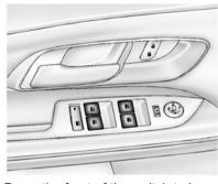
Press the front of the switch to lower the window. Pull the switch up to raise it.
