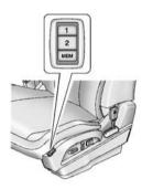
On vehicles with the memory feature, the "1" and "2" buttons on the outboard side of the driver seat are used to manually save and recall the driver seat and outside mirror positions. These manually stored positions are referred to as Button Memory positions.
