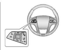
To turn LDW on and off, press the LANE DEPART button, located on the steering wheel.
