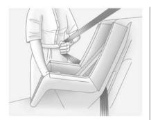
Pull the shoulder belt all the way out of the retractor to set the lock. When the retractor lock is set, the belt can be tightened but not pulled out of the retractor.
