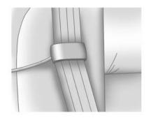
3. The belt should not be twisted and it should lie flat. The elastic cord must be under the belt and the guide on top.
