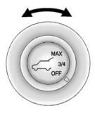
On vehicles with a power liftgate, the switch is on the overhead console. The vehicle must be in P (Park) to use the power feature. The taillamps flash when the power liftgate moves.
