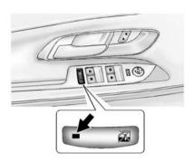
(Window Lockout): This feature prevents the rear passenger windows from operating, except from the driver position.
