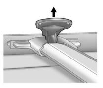
Lift the lever to release and move the cross rail.
