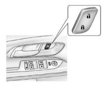
There are power door lock switches on the front door panels.
