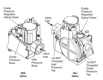
Figure 4 Pressure port and regulator adjust locations
