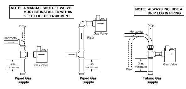
Figure 2. Typical gas valve piping
