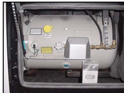
Figure 2-5. Liquid Propane Tank
