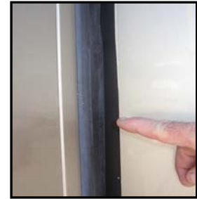
Figure 14-6. Inspecting Slide Out Gasket
