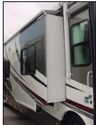
Figure 8-2. Typical Slide-Out Fully Extended
