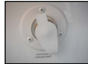
Figure 11-6. City Water Inlet
