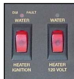
Figure 4-16. Water Heater Switches
