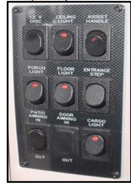
Figure 9-8. Entrance Step Switch (right middle)
