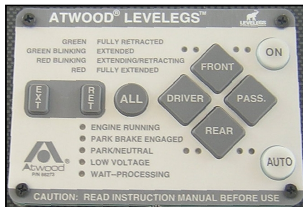
Figure 9-6. Leveling Control Panel on Dashboard
