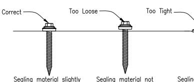
Sealing material slightly visible at edge of metal washer. Assembly is weather tight.
