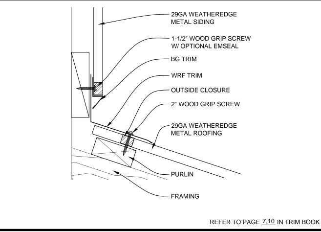
WALL TO ROOF FLASHING
