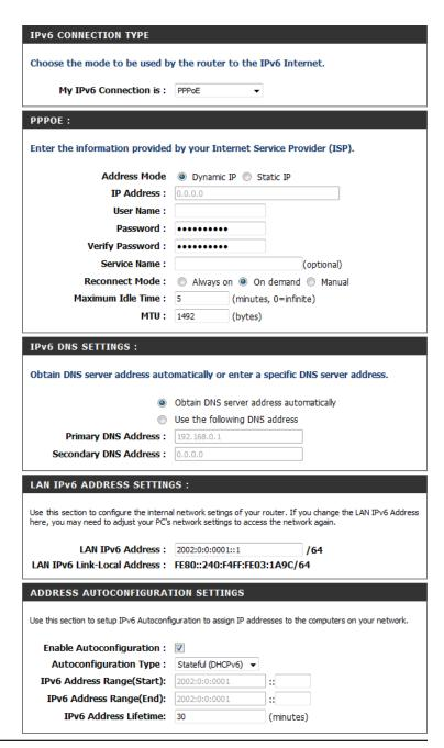
**Enable Autoconfiguration:** Check to enable the Autoconfiguration feature.
