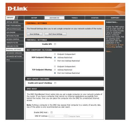
**Note:** Placing a computer in the DMZ may expose that computer to a variety of security risks. Use of this option is only recommended as a last resort.
