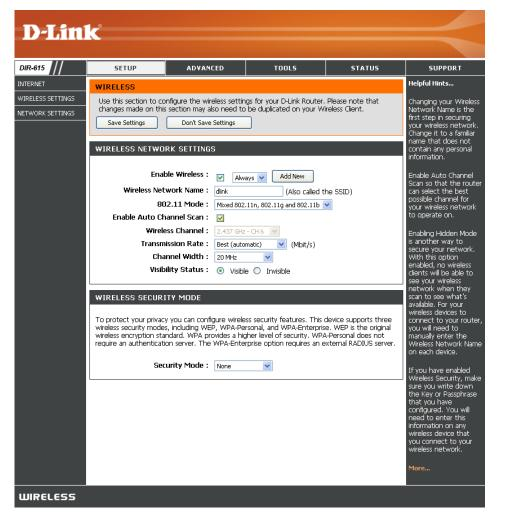
Wireless Channel: Indicates the channel setting for the DIR-615. By default the channel is set to 6. The Channel can be changed to fit the channel setting for an existing wireless network or to customize the wireless network. If you enable **Auto Channel Scan**, this option will be greved out.
