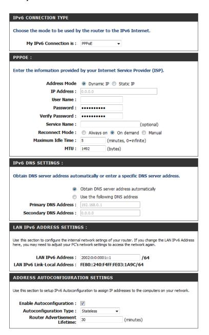
**Enable Autoconfiguration:** Check to enable the Autoconfiguration feature.
