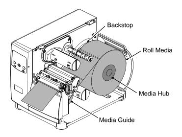
B. Route the Media under the Media Idler, through the Media Sensor, and then straight out the front of printer.
