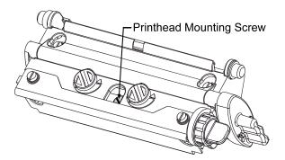
D. Rotate the printhead latch forward and, while supporting the Printhead, raise the Printhead Assembly. Disconnect the Cables and then remove the Printhead.
