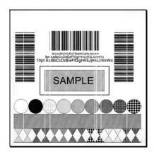
*I* Note: Streaks can indicate a dirty or faulty printhead.
