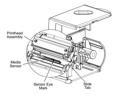
*Notes:* (1) For SENSOR TYPE selection, see Section 4.2.2 (and if using CONTINUOUS also set LABEL LENGTH).
