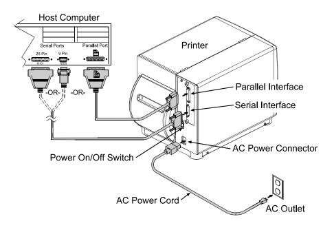
*Note:* When interfacing, ensure AC power has been turned OFF, and always apply power to the Host before the Printer.
