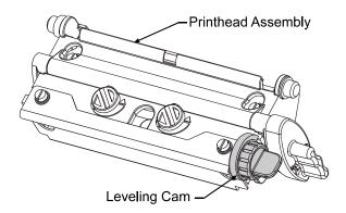
C. Rotate the Leveling Cam clockwise, one click at a time, until the printed labels contain a complete, even image (see Example 2).
