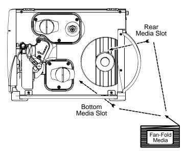
B. Route the Media under the Media Idler (also, if equipped over the Internal Rewinder; and, if through the Rear Media Slot, over the Media Hub).
