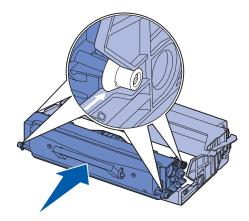
6 Install the toner cartridge assembly into the printer by aligning the green arrows on the guides of the toner cartridge assembly with the green arrows on the tracks in the printer and pushing the toner cartridge assembly in as far as it will go.
