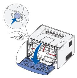
2 Remove the English operator panel by pressing the tab and lifting the panel up.
