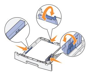
If you are loading legal or folio size paper, press down on the latch at the back of the tray and expand the tray until the extender locks into place.
