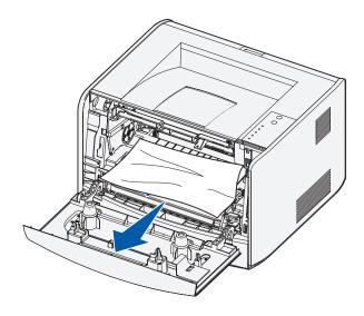
**4** Lift the flap at the front of the printer and remove any jams beneath the flap.
