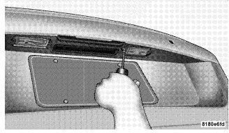
2. Rotate the socket 1/4 turn counterclockwise.
