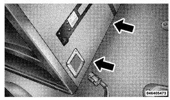
3. Open the liftgate and remove the subwoofer.
