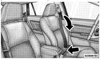
Inserting Latch Plate Into Buckle
