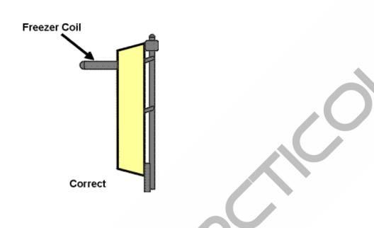
In the graphics below, the is a metal to metal contact point that requires thermal mastic. The where the cooling unit has to make good, snug contact with the refrigerator box.
