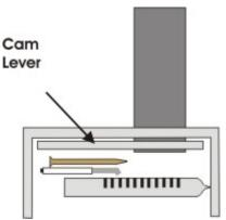
RM1300, RM1301, RM1302, and RM1303 have a cam holding the burner assembly to the bottom of the cooling unit chimney. Locate the cam and pull it's lever towards you (see below). This will allow the burner to drop down. Anything else in the way of pulling the cooling unit needs to be removed.
