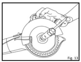
2. Open lower guard and place "Face 2" blade on saw and fit on the outer arbor shaft . (Fig. 10)
