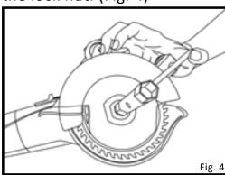
3. Remove lock nut and washer from the blade (fig. 5)
