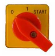
After installation of the mains electric supply, turn the main switch (1) to position 1. This will activate the back gauge motor circuit and the back gauge will move backward to the rear and stop, and recalibrate the position. The cut line light shows and the digital display glows.
