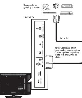
3 Connect the other end of the cable to the AV1 jack and the AV1 audio in jacks on the side of your TV.
