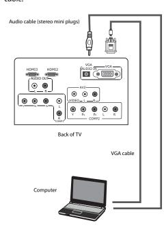
3 Connect an audio cable to the AUDIO OUT jack on the computer, then connect the other end of the cable to the VGA AUDIO IN jack on the back of your TV.
