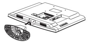
3 Align the base with the bottom of the TV, then secure the base to the TV with the four M6XL 16 mm screws provided.
