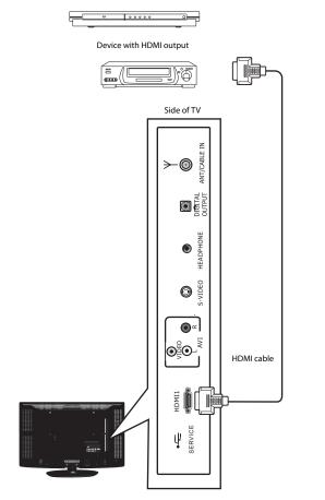
3 Connect the other end of the cable to the HDMI1 on the side of your TV or the HDMI2 or HDMI3 jack on the back of your TV.
