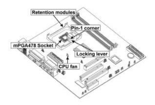
**Note:** The pin-1 corner is marked with an arrow **▶**
