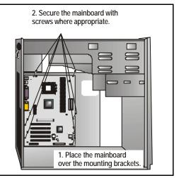
Ensure that your case has an I/O template that supports the I/O ports and expansion slots on your mainboard.
