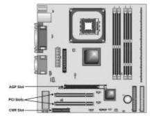
**Note:** Before installing an add-on card, check the documentation for the card carefully. If the card is not Plug and Play, you may have to manually configure the card before installation.
