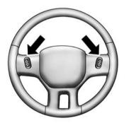
The left-hand control is also a rocker type switch with a push-button in the center. Push the top of the switch to Scan Up  $\Delta$ . Push the bottom of the switch to Scan Down  $\nabla$ . The button in the center is the **PRESET**  $\bullet$ UP/OK button.
