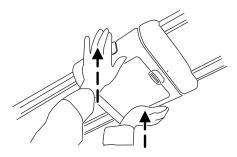
While pushing upwards with palms, grip the side latches with fingers and squeeze.
