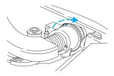
2. Carefully separate the two halves of the air filter housing.
