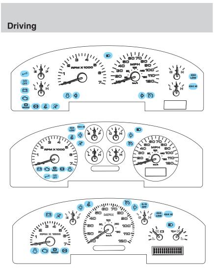
Make sure the corresponding lights illuminate or illuminate briefly. If a light fails to illuminate, have the vehicle serviced.
