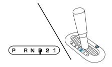
Overdrive can be deactivated by pressing the transmission control switch on the end of the gearshift lever (column-shift transmission) or on the gearshift bezel (floor-shift transmission).
