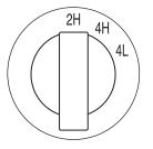
**2H (2WD High)** - Power to the rear wheels only; used for street and highway driving. Provides optimal smoothness and fuel economy at high speeds.
