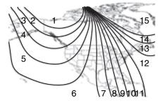
4. Press the ODO reset button in the cluster, hold for six seconds and release. You will see that ZONE appears in the instrument cluster display.
