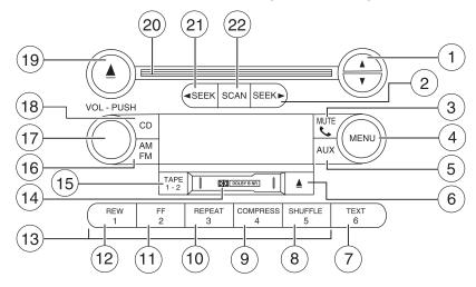
1.  $\blacktriangle$  / **V** Tune: Press to manually go up or down the radio frequency. Also use in menu mode to select various settings.
