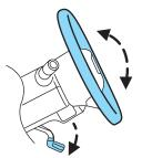
While holding the steering column, pull the lever up to its original position to lock the steering column.
