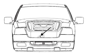
2. Go to the front of the vehicle and release the auxiliary latch that is located on the front bumper under the grill.
