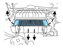
2. Pull air filter tray assembly out toward front of vehicle and lift air filter element up and out of housing.
