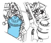
1. Start the engine and let it run until it reaches normal operating temperature (the engine coolant temperature gauge indicator will be near the center of the normal area between H and C).
