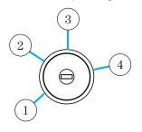
ignition from the 1 (OFF/LOCK) position to the 3 (ON) position (maintain ignition in the 3 (ON) position for at least one second, but no more than ten seconds). This step will program your new key to a coded key.
