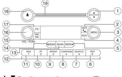
1. A / **Tune:** Press to manually go up or down the radio frequency. Also use in menu mode to select various settings.
