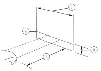
3. Turn on the low beam headlamps to illuminate the wall or screen and open the hood. Cover one of the headlamps so no light hits the wall.
