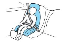
Both can be used in any vehicle in a seating position equipped with lap/shoulder belts if your child is over 40 lbs (18 kg).
