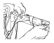
2. Route the tether strap behind the head restraint supports to a loop behind an adjacent seating position, and hook the strap hook onto the loop. If using the driver's side, pass the strap behind the shoulder belt mounting for the center seat.
