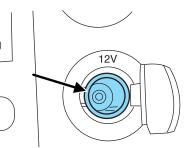
The auxiliary power point is located on the instrument panel.
