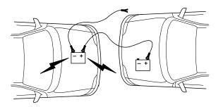
3. Connect the negative (-) cable to the negative (-) terminal of the assisting battery.
