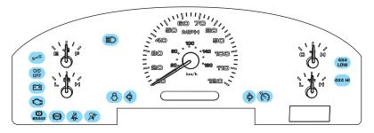
Base with Tachometer instrument cluster
