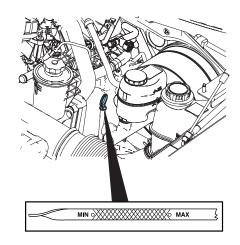
5. Locate and carefully remove the engine oil level indicator (dipstick).
