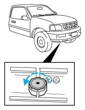
3. Fluid level should be at bottom of the opening.
