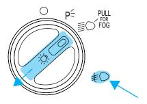
The Daytime Running Light (DRL) system will not illuminate the tail lamps and parking lamps. Turn on your headlamps at dusk. Failure to do so may result in a collision.
