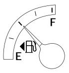
When refueling the vehicle from empty indication, the amount of fuel that can be added will be less than the advertised capacity due to the reserve fuel.
