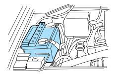
the electrolyte in each cell up to the "level" indicator. Do not overfill the battery cells.
