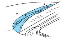
• When placing objects on top of your instrument panel, be careful to not place them over the defroster outlets. These objects can block airflow and reduce your ability to see through your windshield. Also, avoid placing small objects on top of your instrument panel. These objects can fall down into the defroster outlets and block airflow and possibly damage your climate control system.
