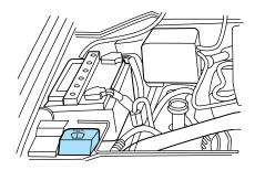
Do not put engine coolant in the container for the windshield washer fluid.
