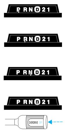
control switch on the end of the gearshift lever.
