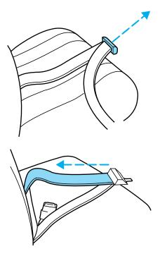
belt. Manufacturer identification is located at the end of the webbing on the label. Also, use the safety belt extension only if the safety belt is too short for you when fully extended. Do not use extensions to change the fit of the shoulder belt across the torso.
