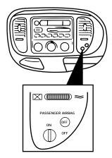
Keep the passenger air bag turned on unless there is a child seat installed in the front seat. When the passenger air bag switch is turned off, the passenger air bag will not inflate in a collision.
