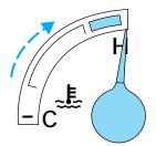
As the engine temperature cools, the engine may be re-started. Take your vehicle to a service facility as soon as possible to minimize engine damage.
