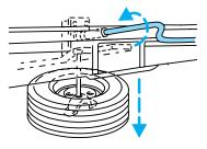
2. Slide the wheel under the vehicle and install the retainer through the wheel center.
