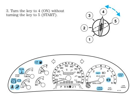
Make sure the corresponding lights illuminate briefly. If a light fails to illuminate, have the vehicle serviced.
