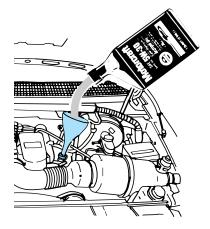
• Oil levels above the MAX mark may cause engine damage. Some
