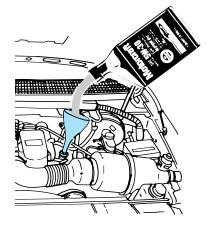
• Oil levels above the MAX mark may cause engine damage. Some oil must be removed from the engine by a service technician.
