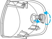
9. Align top and bottom ribs of parking lamp assembly with corresponding slots on front of vehicle.
