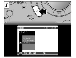
Press the "MENU/OK" button to display the menu on the monitor.
