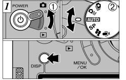
①Set the Mode switch to " **①**" ② Set the Photography Mode dial to " **D O**". For viewfinder photography (other than Macro mode), press the "DISP" button to switch the LCD monitor off.
