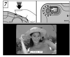
Press the shutter button down half way. The image is focused when the AF frame on the LCD monitor becomes smaller and the shutter speed and aperture setting appear (and the green viewfinder lamp stops blinking and remains lit).
