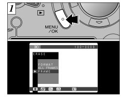
Press the "MENU/OK" button to display the menu on the LCD monitor.
