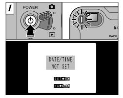
Press the " $\bullet$ " (power) button to switch the camera on and off. When you switch the camera on, the viewfinder lamp lights (green). If the date has been cleared, a confirmation
