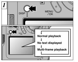
In playback mode, the display shown on the LCD monitor switches each time you press the "DISP" button. Press the "DISP" button until the multi-frame playback screen (9 frames) appears.
