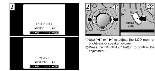
When you use the "LCD BRIGHTNESS" or "VOLUME" settings, an "adjustment bar" appears on the LCD monitor.
