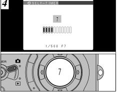
The time until the shutter releases is shown as a countdown bar on the LCD monitor and display panel.
