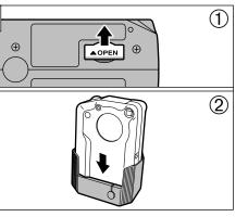
①Open the connection socket cover on the bottom of the camera. <sup>(2)</sup>Switch the camera off and place it in the cradle.
