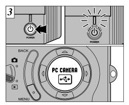
When you press the "O" (power) button on the cradle, the camera is connected to your PC and the power lamp on the cradle lights. "PC CAMERA" also appears on the display panel. • Focal range: Approx. 50 cm (1.6 ft.) to infinity
