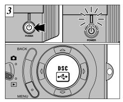
When you press the " $\bullet$ " (power) button on the cradle, the camera is connected to your PC as a removable disk drive and the power lamp on the cradle lights. "DSC" also appears on the display panel.
