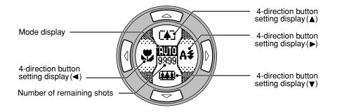
\* The display panel can be used to check and modify camera settings such as the photography or playback mode, the number of available shots, the flash settings and the macro setting.
