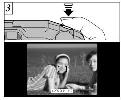
Keep holding the shutter button down halfway (AF/AE lock). Check that the AF frame on the LCD monitor shrinks and that the shutter speed and aperture setting are displayed (the viewfinder lamp (green) changes from blinking to steady).
