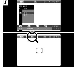
This function can be selected in the " $\mathbf{C} \cdot \mathbf{\Delta}$ M" and " $\mathbf{\Omega}$ " photography modes. When the camera cannot focus in AF mode, use this mode to set the focus and take the picture.
