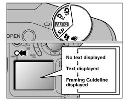
The photography mode can be set to "AUTO  $\cdot$  **SP**  $\cdot$  **D**M or **D**". The mode shown on the LCD monitor switches each time you press the "DISP" button. Press the "DISP" button to display the framing guideline.
