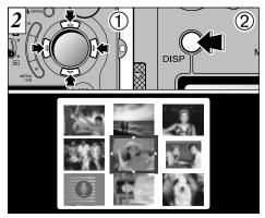
① Select a frame by using "◄", "▶", "▲" and "▼" button to move the cursor (the orange box) to the desired frame. Press the "▲" or "▼" button several times to switch to the previous page or the next page.
