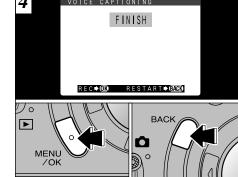
When you have recorded 30 seconds of sound, the "FINISH" message appears on the LCD monitor.
