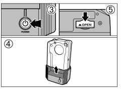
③ Press the "O" (power) button on the cradle and then disconnect the cradle from the PC.
