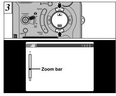
In Movie mode, the lens is locked at the wideangle setting and only the digital zoom can be used. You can use " $\blacktriangle$ " and " $\blacktriangledown$ " to zoom in and out. A "zoom bar" is displayed on the LCD monitor.
