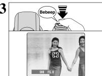
When you press the Shutter button down halfway, the camera emits a short double-beep and focuses on your subject. At that point, the AF frame on the screen becomes smaller and the camera sets the shutter speed and aperture (the indicator lamp (green) changes from blinking to lit.).
