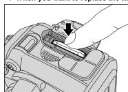
Ensure that the camera is switched off before opening the slot cover. When the **xD-Picture Card** is pushed into the slot and then slowly released, the card lock releases and the **xD-Picture Card** is pushed out.
