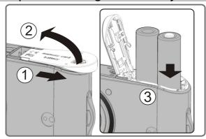
Slide open the battery cover in the direction shown by ① and then lift the cover in direction ② as shown.
