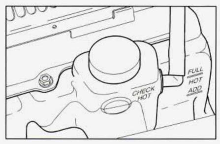
The coolant level should be at least up to the ADD mark.
