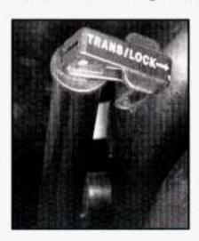
The transmission dipstick has a red handle and is located at the rear of the engine compartment. Flip the handle up and then pull out the dipstick and wipe it with a clean rag or paper towel. Push it back in all the way, wait three seconds and then pull it back out again.
