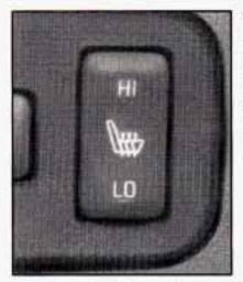
This control is located on the side of the seat. This feature will quickly heat the lower cushion and lower back of the driver and front passenger seats for added comfort.
