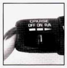
3 Press in the SET button at the end of the lever and release it.
