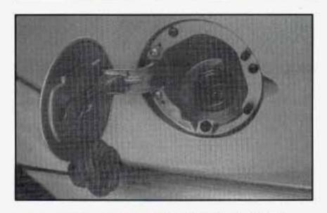
While refueling, hang the cap by the tether from the hook on the filler door. To remove the cap, turn it slowly to the left (counterclockwise). The cap has a spring in it; if you let go of the cap too soon, it will spring back to the right.
