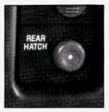
This button on the passenger's side of the steering column allows you to release the liftglass from inside the vehicle.
