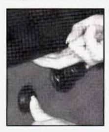
To open the liftglass only, press the button and pull up on the handle.
