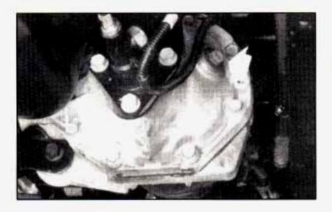
If the level is below the bottom of the filler plug hole, you may need to add some lubricant. When the differential is cold, add enough lubricant to raise the level to 1/2 inch (12 mm) below the filler plug hole.
