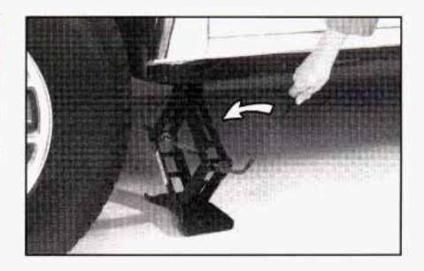
9. Lower the vehicle by turning the jack handle to the left. Lower the jack completely.
