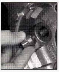
Put the nuts on by hand. Make sure the cone-shaped end is toward the wheel.
