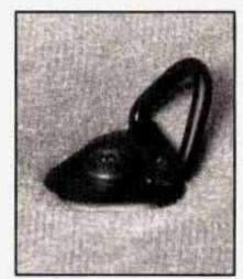
There are four cargo tie downs in the rear that allow you to strap cargo in and keep it from moving inside the vehicle.
