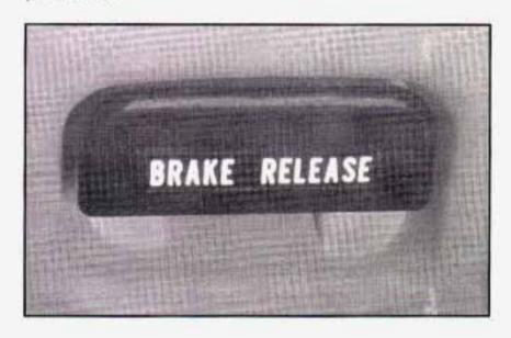
Pull the BRAKE RELEASE lever. It is located on the bottom of the driver's side of the instrument panel.
