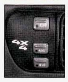
The transfer case switches are above the radio controls.
