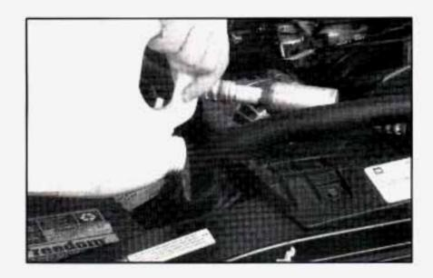
Fill the radiator with the proper DEX-COOL<sup>®</sup>
