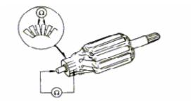
inspection for electric conduction capability of armature
