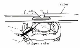
inspection for distortion of cylinder
