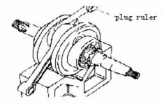
crankshaft and connecting rod inspection
