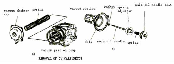
For plug throttle its structure is the following figure: after removing it, inspect whether its fluctuating movement is smooth and main oil needle is abraded or not.
