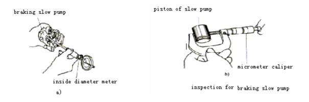
Disassembled configuratin of braking main pump as shown, inspect its body and piston after disassembling it including damage, scratch and step abrasion on its surface, and replace them if necessary. Measure main pump's inside diameter for several times with centesimal meter and measure the outside diameter of piston of main pump for several times with micrometer as shown. If one diameter is out of its limit, replace it.
