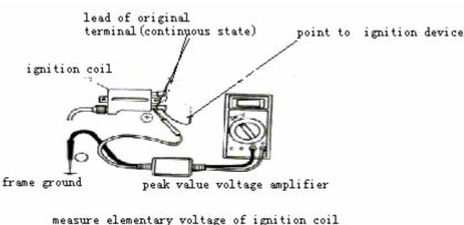
When using peak votage to inspect ignition coil, take down plug from CDI device and connect the end of ignition coil with leak voltage amplifier. If the gap of spark plug is proper, turn crankshaft through starting motor, and then read the leak voltage of ignition coil.
