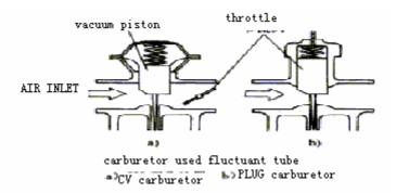
For PLUG carburetor, throttle handle grip control throttle to get your required operation (see fig.).
