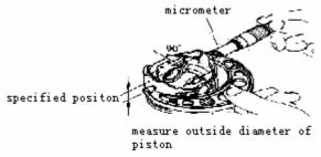
Inspect the hole of piston pin (see fig.): measure it in direction X AND Y, regard the maximum as its inside diameter. Replace it if the maximum is over its limit.
