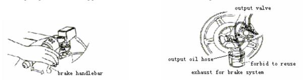
Replace braking liquid following as the above figure. Remove main pump cover and
