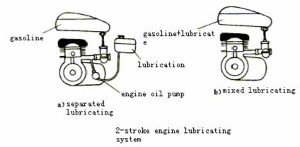
Engine oil pump is main part of lubricating device, for 4-stroke engine its engine oil pump uses trochoid gear pump and for 2-stroke engien it uses plug enginge pump.
