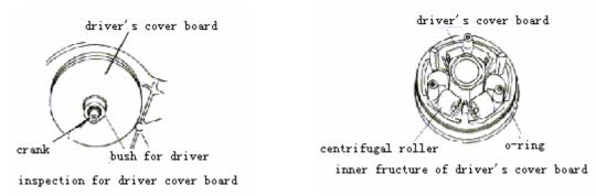
Insepct driver's centrifugal roller, cover board and bush (see fig.). If damaged or declining abraded, replace it. Measure outside diameter of centrifugal roller and bush, inside diameter of cover board.replace it if measured diameter is over its limit.
