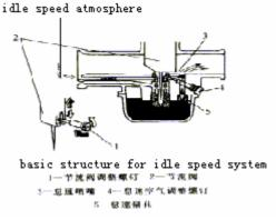
For idle speed system it makes use of negative pressure resulted from engine operation to spray fuel from idle speed nozzle, which ensures the supplement of fuel. Commonly, there are throttle djusting screw and idle speed atmosphere screw. Throttle notch screw adjusts the lest open of throttle, and idle speed atmosphere screw adusts fuel capacity mixed atmosphere which is controlled by idle speed jet. Idle speed screw adjusts atomized fuel capacity gotten through idle speed jet.
