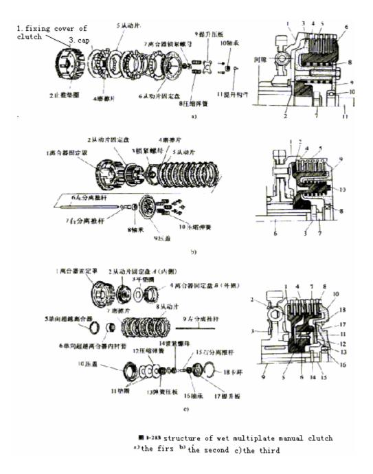
There are two forms for wet multiplate acentric clutch. For the first form its basical structure and the route of drive transmission is the following picture, and for the second form its basical structure is following picture.
