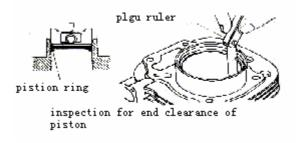
If measured end clearance or side clearance is over its limit, replace piston ring.
