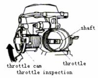
For CV type of carburetor its removal structure is the following figure: after removing it inspect whether vacuum tube can rotate smoothy in carbutetor. Inspect whether there
