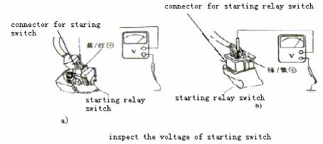
Inspect grounded ciucuit of starting relay switch (see fig.): for the first kind one, inspect whether purple-grounded lead for the plug of starting switch puts through ground well. When transmission is positioned on empty position or when you grasp clutch lever, the grouned lead of relay puts through ground well, that means that this ciruit diagram is good. For the second kind one, inspection is essentially the same of the inspection for the first kind one.
