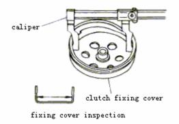
Measure outside diameter of driven wheel and the touching part of driven left disc, replace it if measured diameter is below its limit. Measure inside diameter of driven wheel left disc; replace it if measured diameter is below its limit. Inspect guide pin groove on driven wheel disc; replace it if abrasion like side step appears.
