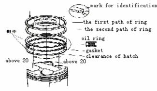
piston ring assembly for four-stroke engine
