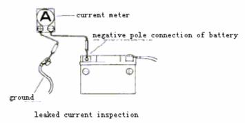
If charge is not ideal, inspect the status with engine warmed up (see fig.); place the battery on vehicle (for opening kind of battery with connection whose voltage is above 13.0v and density of electrolyte is 1.27cm3 ( $20^{\circ}$ C)). Assemble digital voltage meter between between connections of
