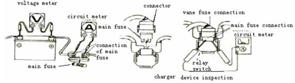
Electric adjustive voltage/rectifier are main charge device, inspect insulation of lead connector and its capability. To inspect insulation of lead connector, remove electric adjustive voltage/rectifier; make use of main lead connector to inspect its insulation (see fig.).
