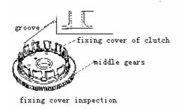
Bush of clutch fixing cover and bearing: if measured inside diameter of bush of clutch fixing cover or its outside diameter is over or below its limit dimension, replace it.
