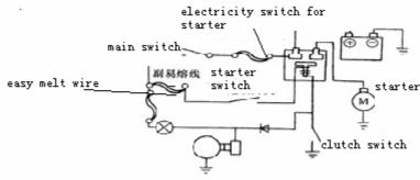
operation principle for clutch switch
