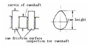
Including the following outer dimension: outside diameter of axes cervix, height of
