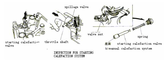
For throttle, you also need to inspect whether moving shaft becomes flexible or not, pull spillage valve of throttle with finger to inspect whether it can be opened or closed. For manual starting concentration valve, you also need to disassemble it and inspect its surface, if there is damage, leaning abrasion or sidestep fray on the seat of valve, replace it.
