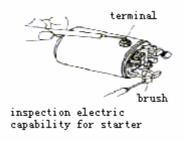
Measure the distance of brush (see fig.), inspect whether the degree of abrasion is over its limit or not, replace it if it is.
