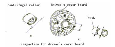
More disassembled removed clutch and driven wheel, compress cluth and driven wheel with clutch pinchcock, fix the clutch pinchcock on table vice, remove lucknut with locknut wrench, and remove pinchcock, clutch and spring (see fig.): remove seal bush and guide pin, then remove the left disc of driven wheel.
