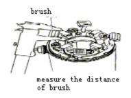
Do some necessary inspections for armature commutator, replace it if the surface is not even, damaged or burnt. See the following picture, and inspect electri conduction capability of armature. It is normal for electric conduction between vanes of commutator and for unable electric conduction between vanes of commutator and armature.
