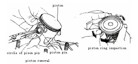
When inspecting piston and piston ring, first of all clean out carbon deposit. It is admitted to use old piston ring to do it. Never use steel wire brush to clean out them, otherwise it may damage its groove. Inspect the top and bottom surface of pison ring groove, replace piston if any damage or wry sharpennig appears (see fig.).
