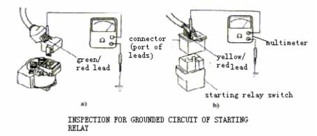
Assemble storage battery on the two ends of terminal of relay switch plug to inspect the electricity conduction between the terminal of storage battery and the terminal of starter through multimeter, electricity conducts well if the ohm value is zero, otherwise relay is damaged.
