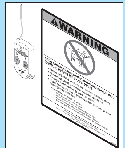
FIG. 3-5 Mounting Entrapment warning label.
