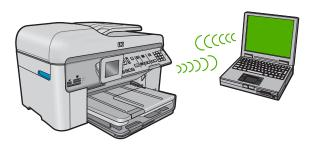
There are two methods you may use to connect the HP Photosmart to your computer using an ad hoc wireless network connection. Once connected, you can install the HP Photosmart software.
