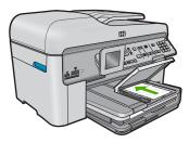
4. Slide the paper-width guide inward until it stops at the edge of the paper. Do not overload the photo tray; make sure the stack of photo paper fits within the photo tray and is no higher than the top of the paper-width guide.
