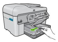
3. Insert the stack of photo paper into the photo tray with the short edge forward and the print side down. Slide the stack of photo paper forward until it stops. If the photo paper you are using has perforated tabs, load the photo paper so that the tabs are closest to you.
