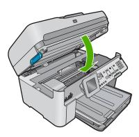
The print carriage is not stalled or blocked. Turn off the product, remove any objects that
